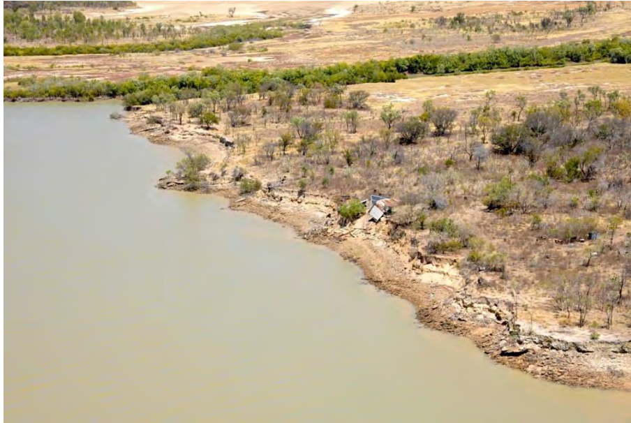
Figure 5.56. Damage from access tracks and bank erosion, notable issues for the Albert.
