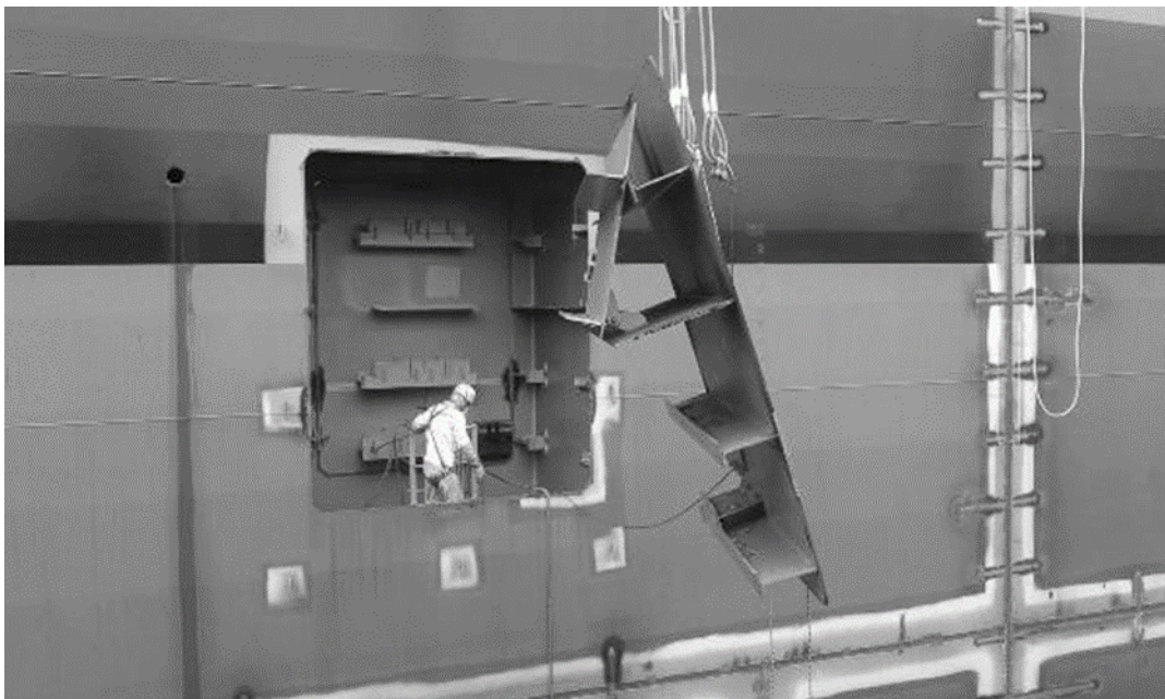
Figure 12. Ship's Hull Being Moved into Place so It Can be Welded from the Inside, South Korea.
