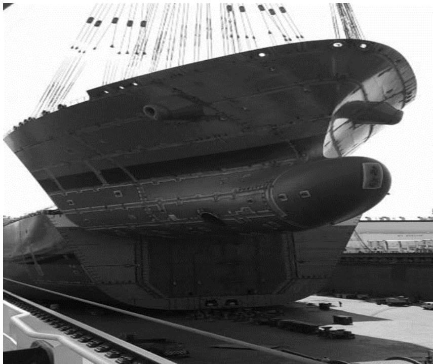
Figure 9. Ship's Bow Being Lowered into Drydock by Sea Crane, South Korea.
