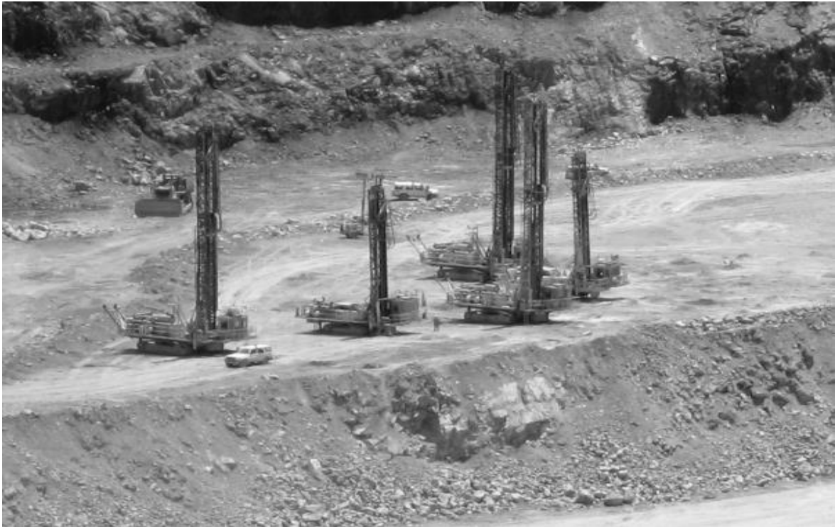
Figure 7. Five Drill Rigs Drilling Holes to House Explosives in an Open Cut Mine, Australia.
