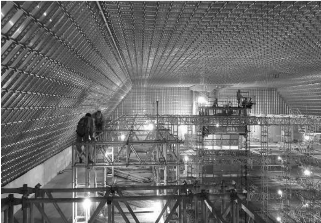
Figure 15. Cargo Hull Scaffolding Being Dismantled by Workers After the Cargo Containment System Has Been Installed, South Korea.
