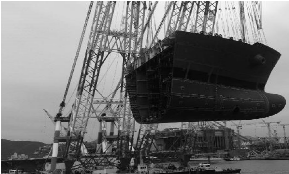
Figure 8. Ship's Bow Lifted into Place by Sea Crane, South Korea.
