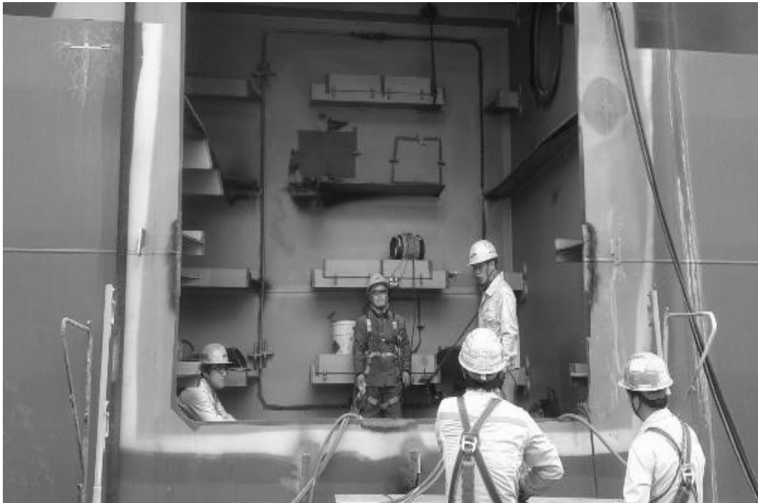
Figure 11. A Welder is Preparing to be Sealed in a Cargo Hull Section to Weld the Inside of the Hull, South Korea.
