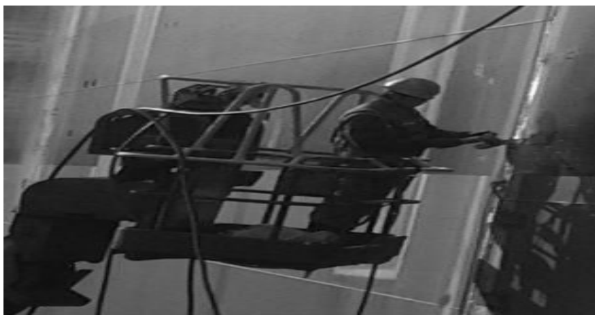
Figure 17. Welder Grinding in an Elevated Work Platform on the Side of a Ship Under Construction, South Korea.
