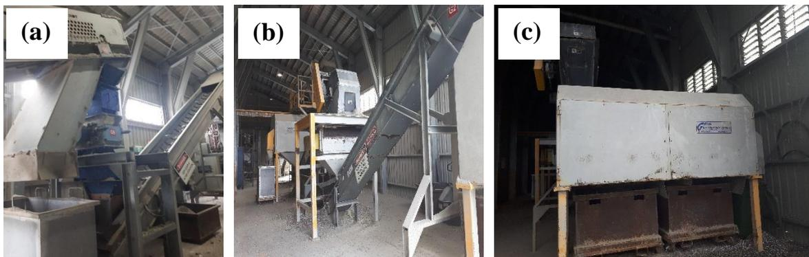
**Figure 3.2 Glass crushing machine (a) imploder (b) shearing unit (c) sanding unit**
