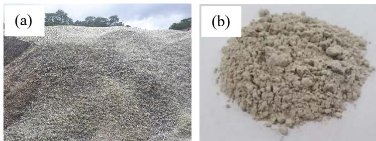
**Figure 4.1 (a) Crushed glass (3 mm size) at MRF site, (b) glass powder (45 µm size)**
