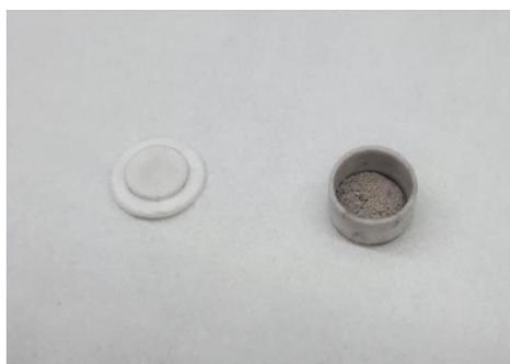
**Figure 5.4 Alumina crucible**
