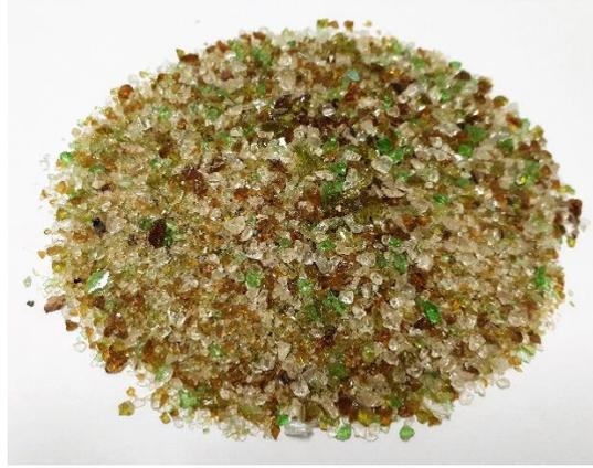
**Figure 3.3 Fine glass sand (3 mm) used as a partial coarse sand replacement**
