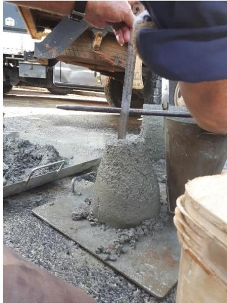
**Figure 7.11 Slump test**
