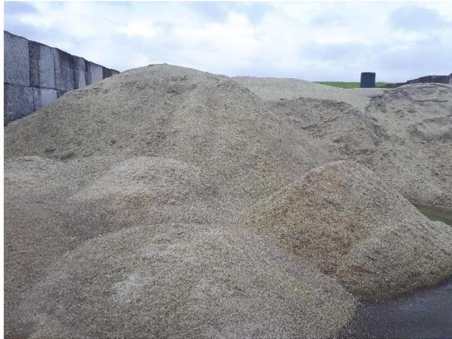
**Figure 7.1 Crushed glass (3 mm size) at MRF site, Cairns**
