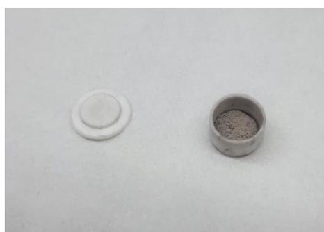
**Figure 5.4 Alumina crucible**
