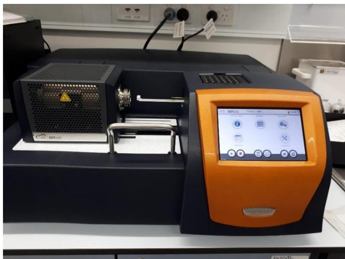
**Figure 5.3 Thermal analyser SDT 650**
