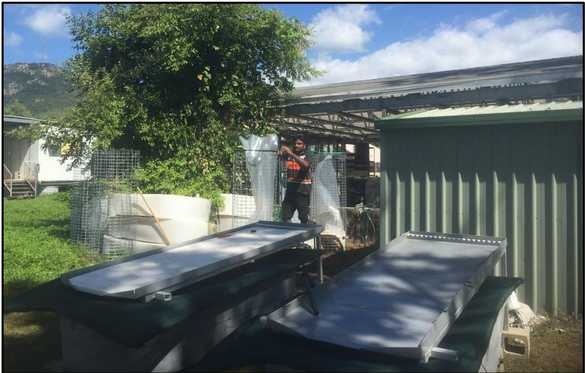
Figure D.2 Wire cage vertical bag systems used in this study for bubbled suspension culture of *Tolypothrix* sp.
