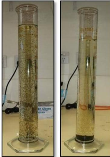
Fig C.3 Images of the self-flocculation behaviour test of *Tolypothrix* sp.
