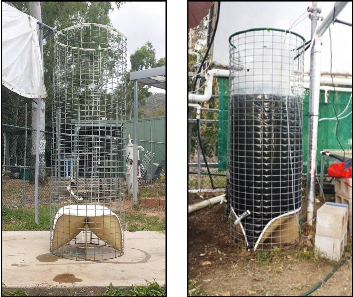
**Figure C.1** Images of the low cost mass production systems used in this study. Left one- Cage used for the vertical bag (suspension culture); Right one- Vertical bag (suspension culture) with 1-week old *Tolypothrix* sp. culture.
