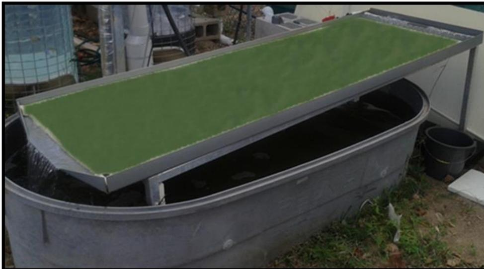
Figure D.1 Modified algal turf-scrubber used in this study for biofilm cultivation of *Tolypothrix* sp.
