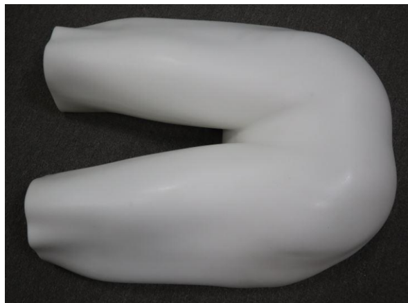
Figure 4. Indenter shell. This picture shows a shell version with a surface layer of soft neoprene, however using the same geometry as the indenter shell in the experiment.
