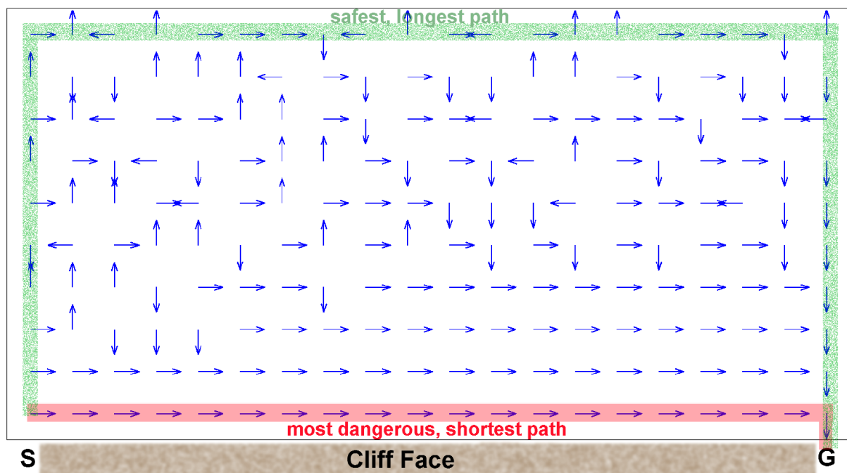
Figure 1: The cliff-walking problem. Q -learning under nondeterministic action-selection found a risky solution.
