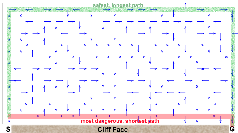
Figure 4: Heger's \hat{Q} -learning under nondeterministic state-transitions shows its extreme pessimism. The player jumps off the cliff from the start square to avoid the higher total cost of falling later.
