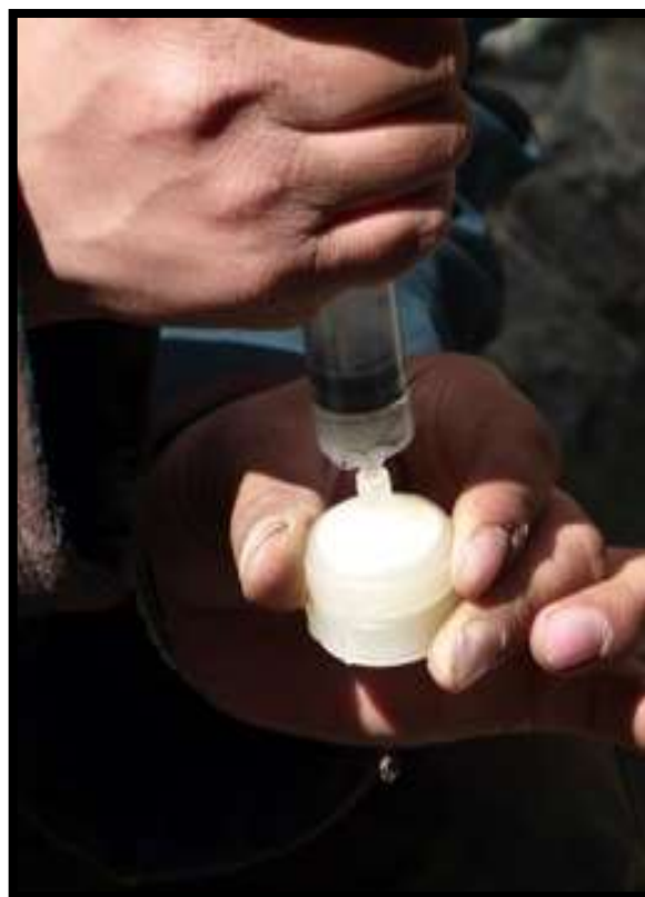
Plate 5.5 Filtering of water through a sterivex filter.
