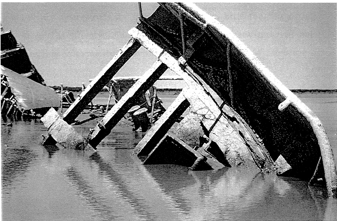
69c: The stern, showing the integrity of the section in comparison with the cargo-hold.
