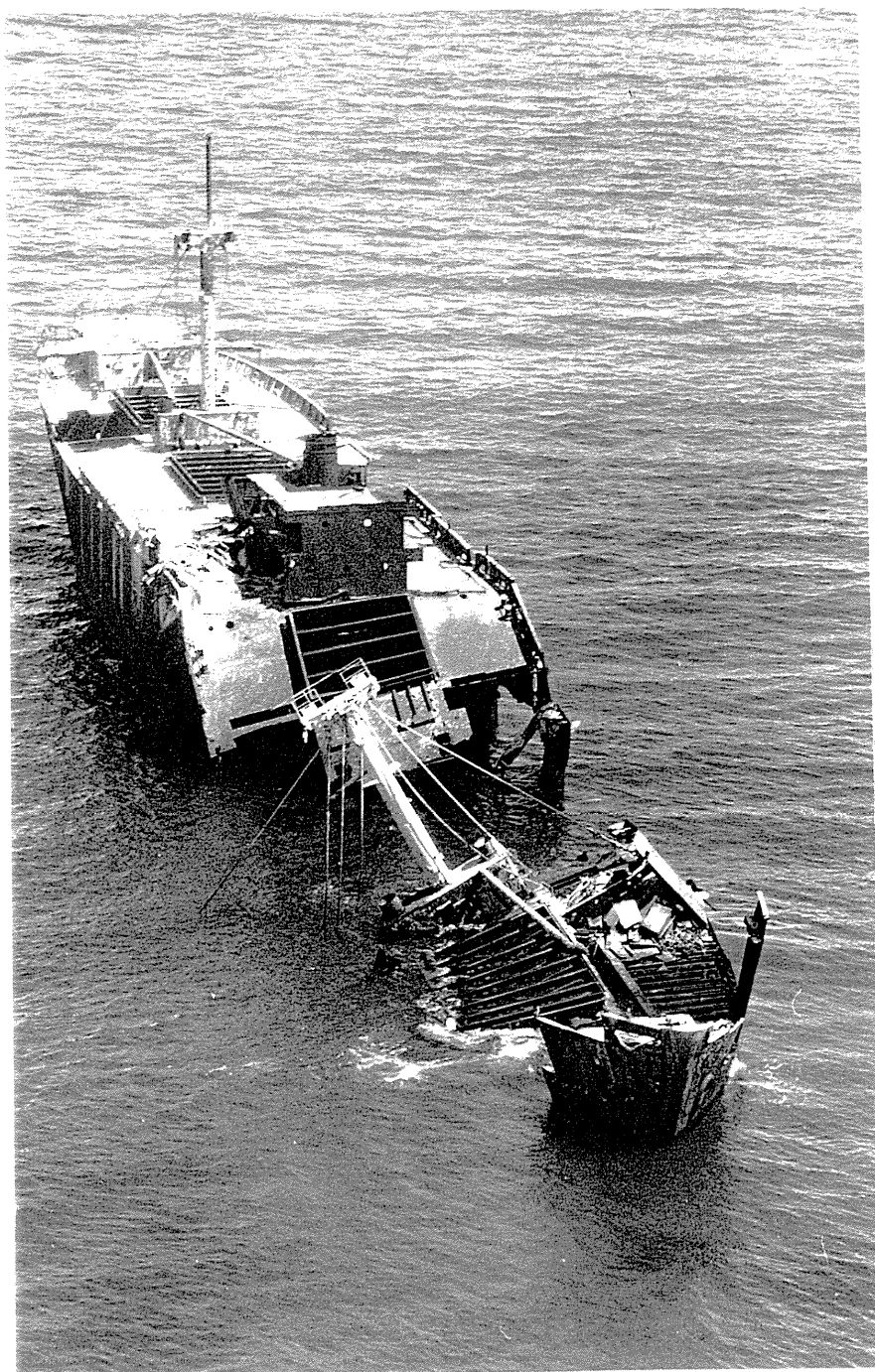
Figure 71: An aerial view of SS Alkimos showing the collapse of the forward cargo hold. Photo by R. Gould, 1995.
