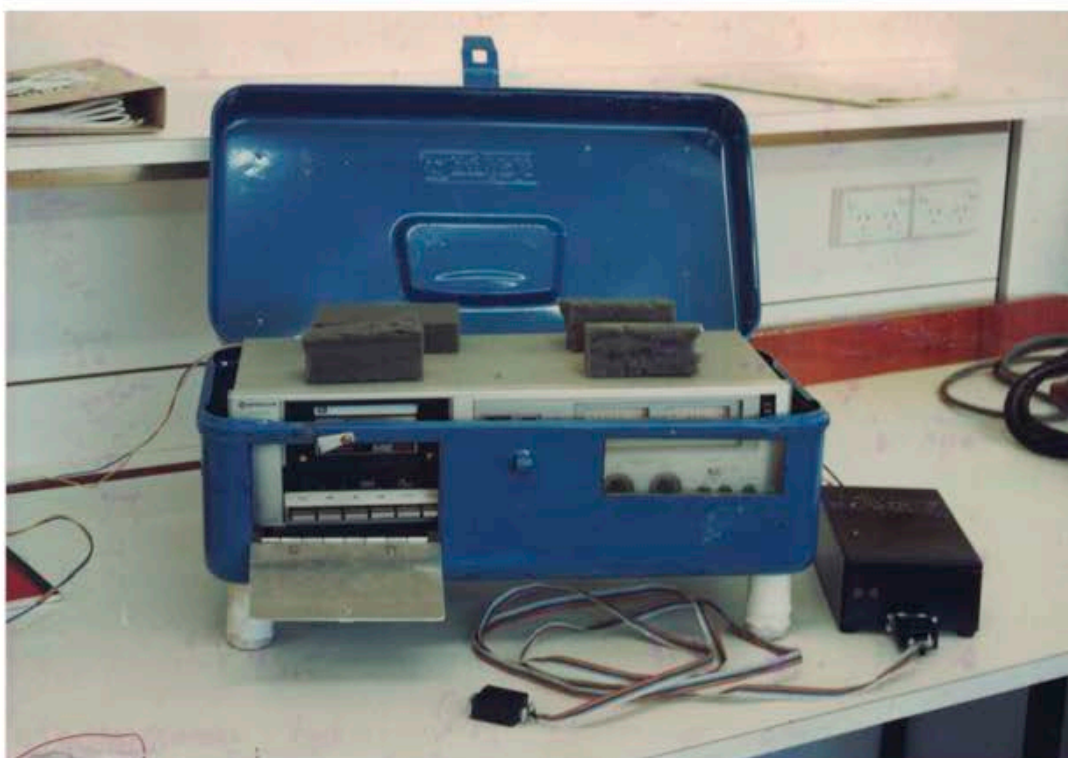
Figure 18 Cassette Tape Deck in foam lined tool box with Interface Electronics at right
