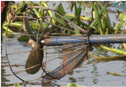
Figure 10.1. Propeller guards designed to be used on boats while dolphin-watching.
