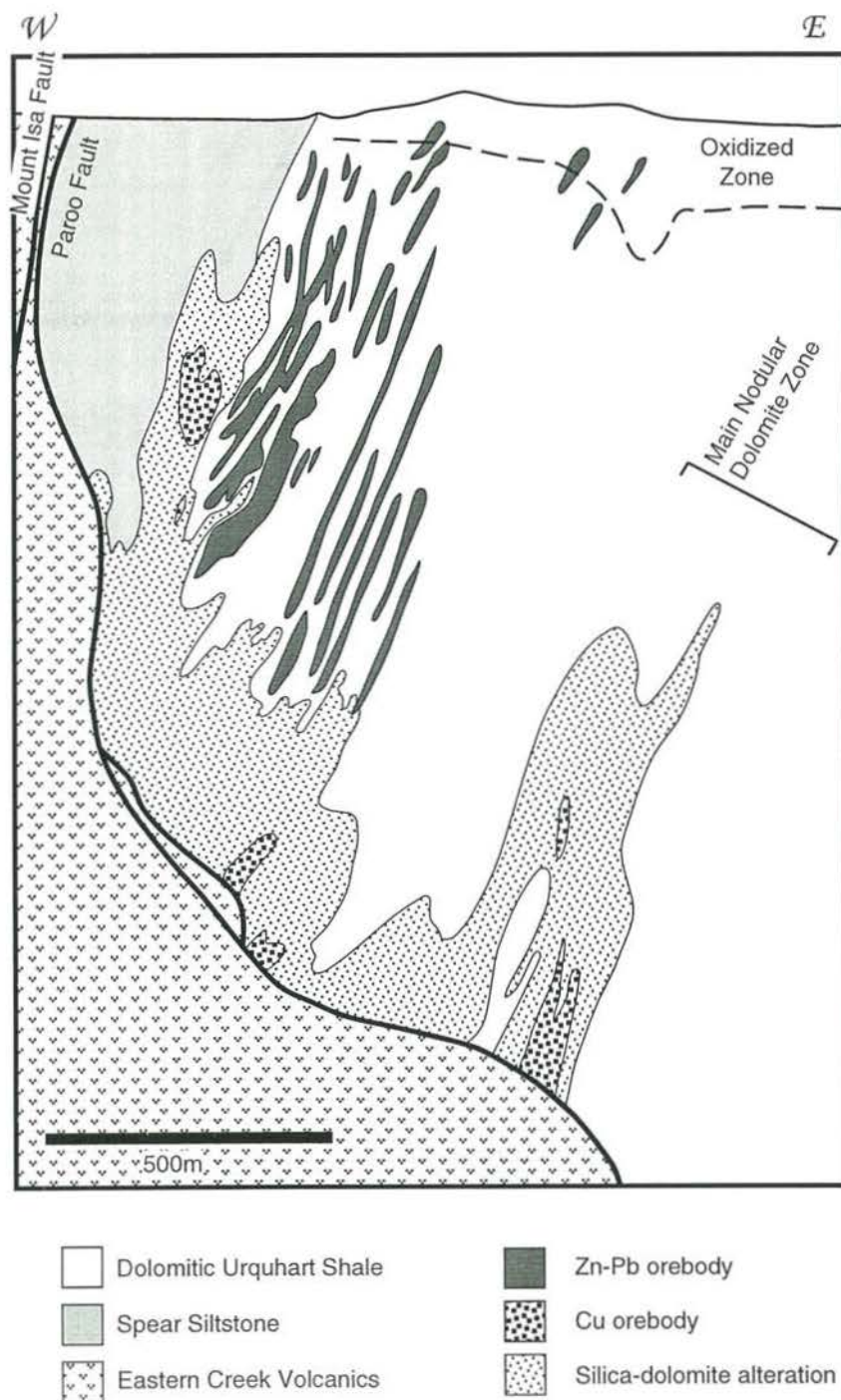
Figure 4. Simplified northern cross-section of Mount Isa Mine illustrating large-scale distribution of Cu and Zn-Pb mineralization, and nodular dolomite - rich portions of stratigraphy in otherwise ferroan dolomite-bearing Urquhart Shale (after Perkins, 1997).
