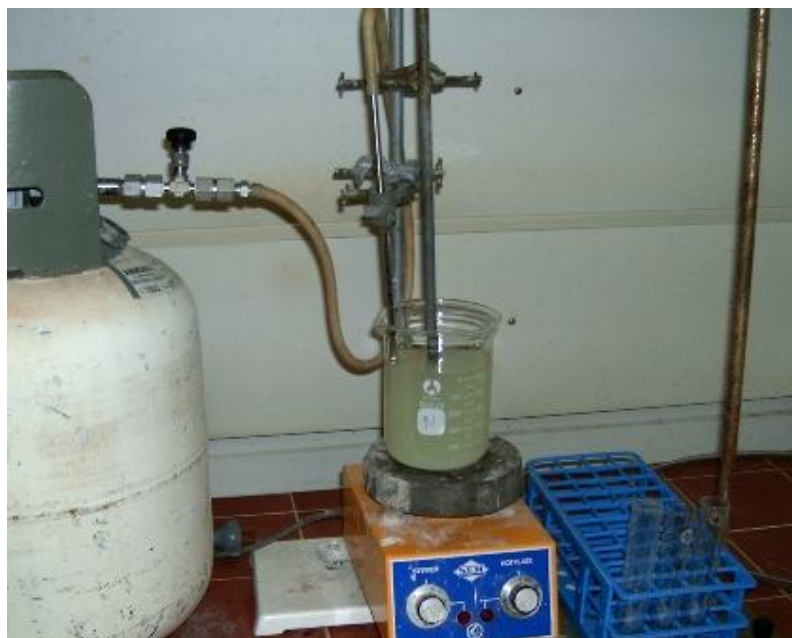
Figure 15: Experimental Apparatus Used To Ammoniate The Phosphoric Acid.
