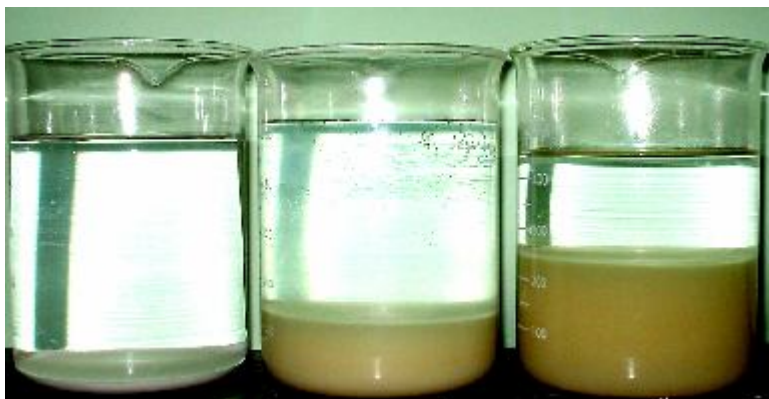
Figure 57: 30ml Of Slurry Settled After Stirring With 500 ml Of Water At Three Different Mole Ratios. Increasing Mole Ratio Shows Resultant Suspended Solids Layer Increasing In Volume And Progressively Darkening To Yellow.
