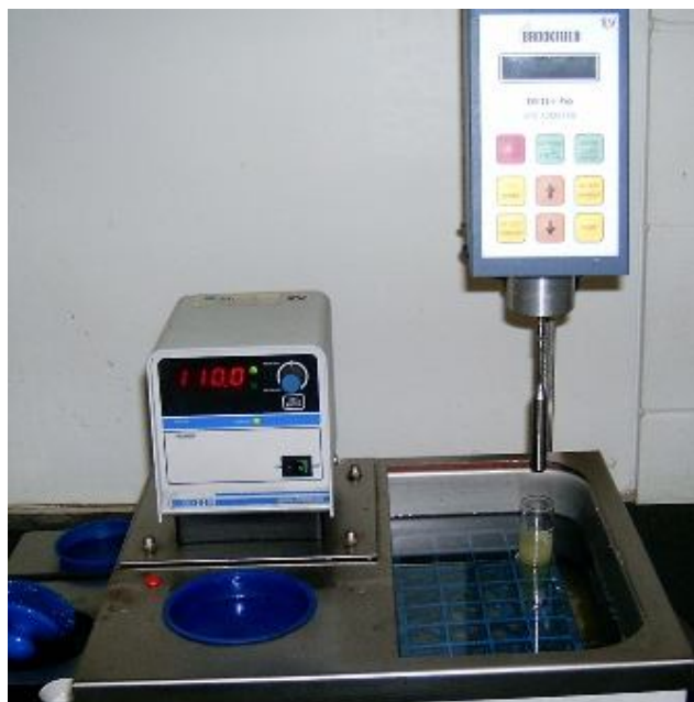
Figure 16: Experimental Apparatus Used To Test For Viscosity.
