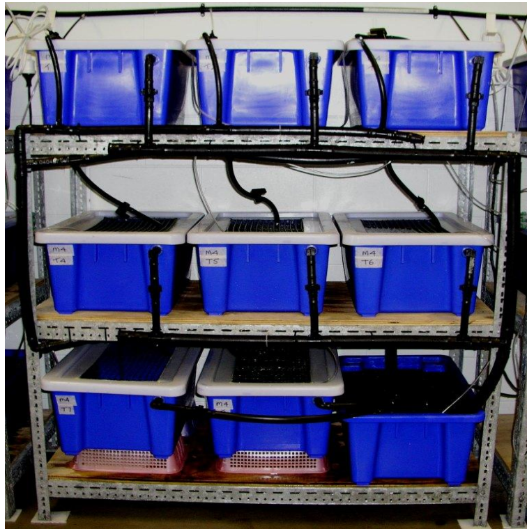
Figure 3.1: Holding and experimental system showing one complete module consisting of nine, 50L tanks, eight tanks for holding animals and one tank used as a biological filter (bottom right tank).
