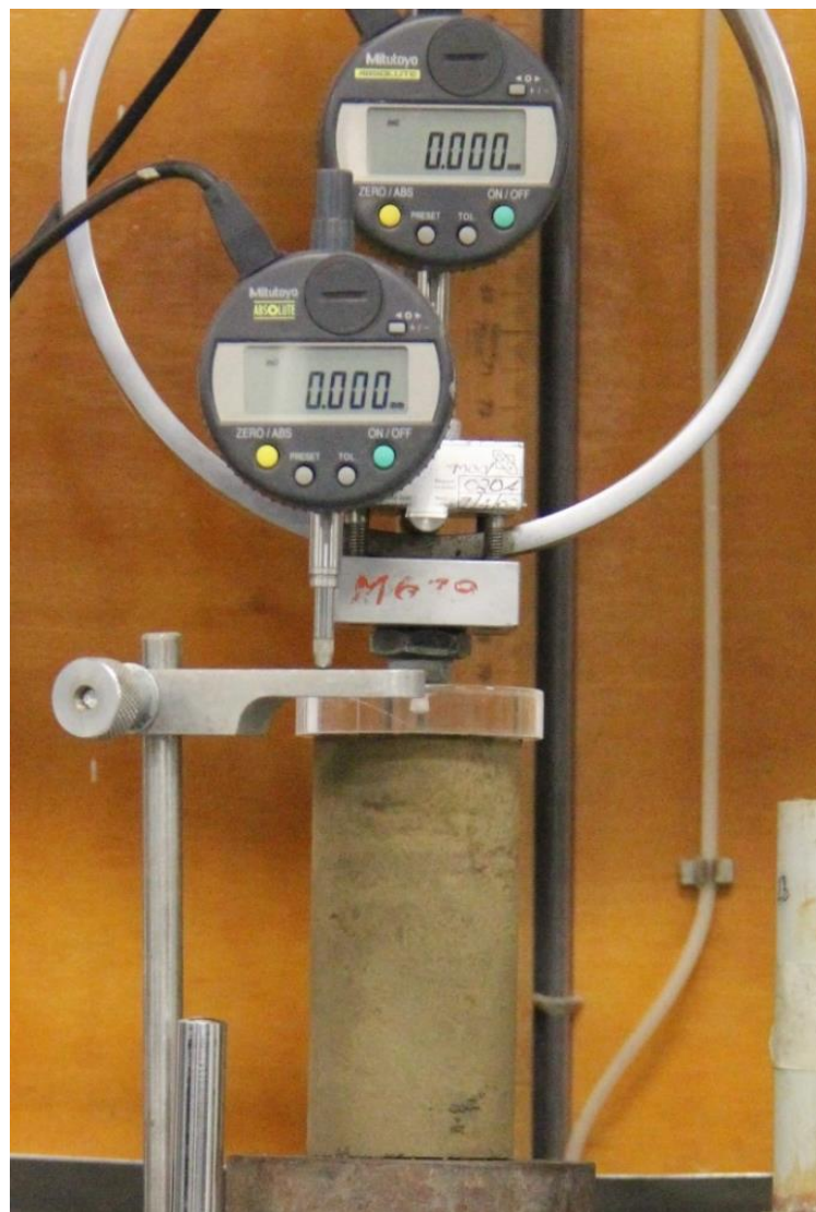
Fig. 6.6 A cemented paste backfill (CPB) sample in UCS test setup
