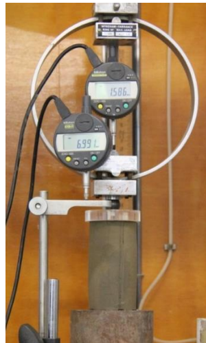
Fig. 8.1 Experimental setup for UCS test of CPB sample
