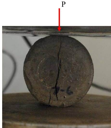
Fig. 8.3 Experimental setup for an IDT strength test of cylindrical CPB sample
