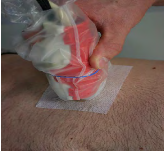
Plate 8.1. The ‘force probe device’ attached to the real-time ultrasound probe and standardised position using adhesive template.
