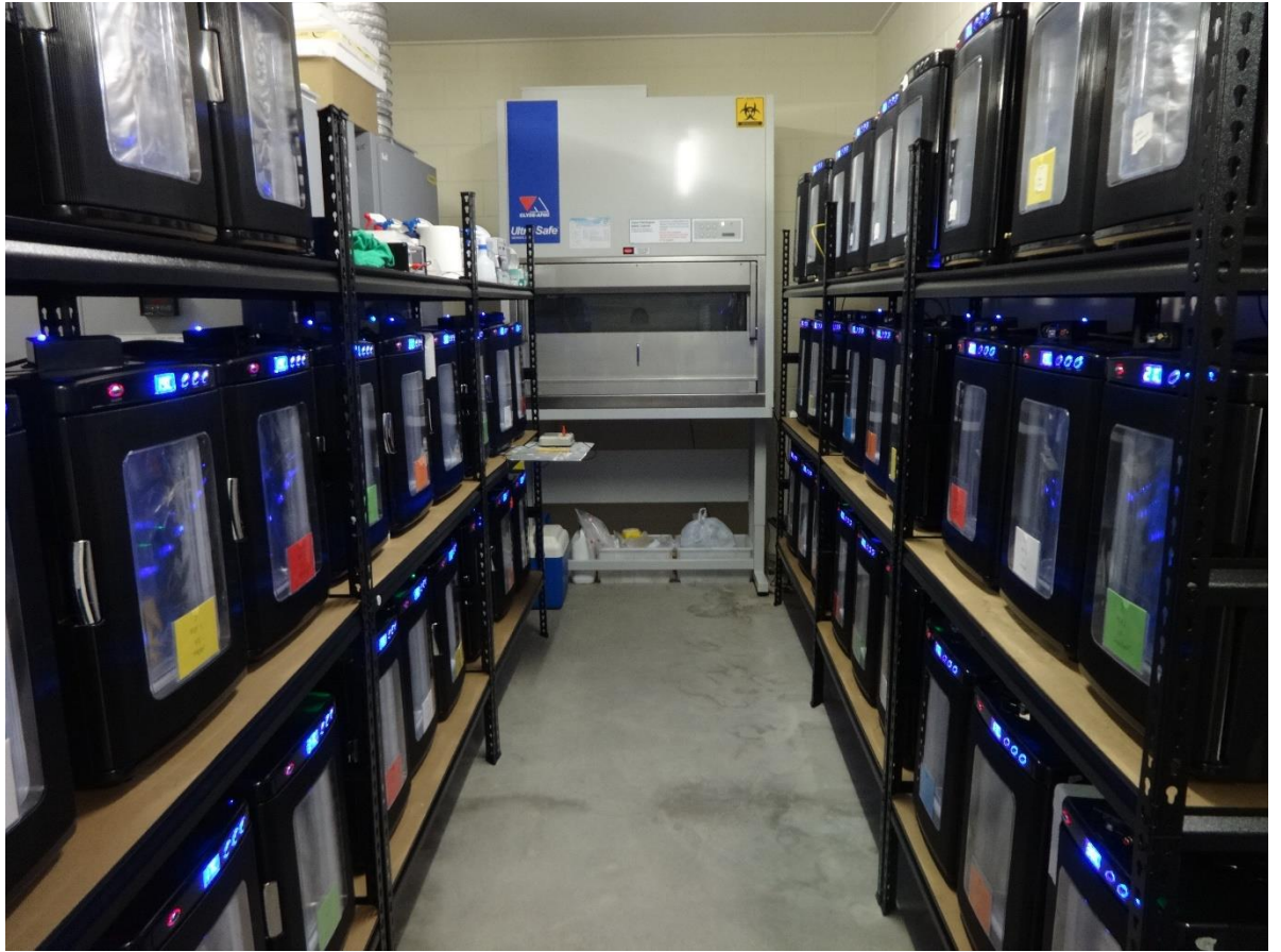
Figure 2.7 Laboratory setup with 48 economical, fluctuating-temperature chambers, each operated by an Arduino UNO microcontroller.
