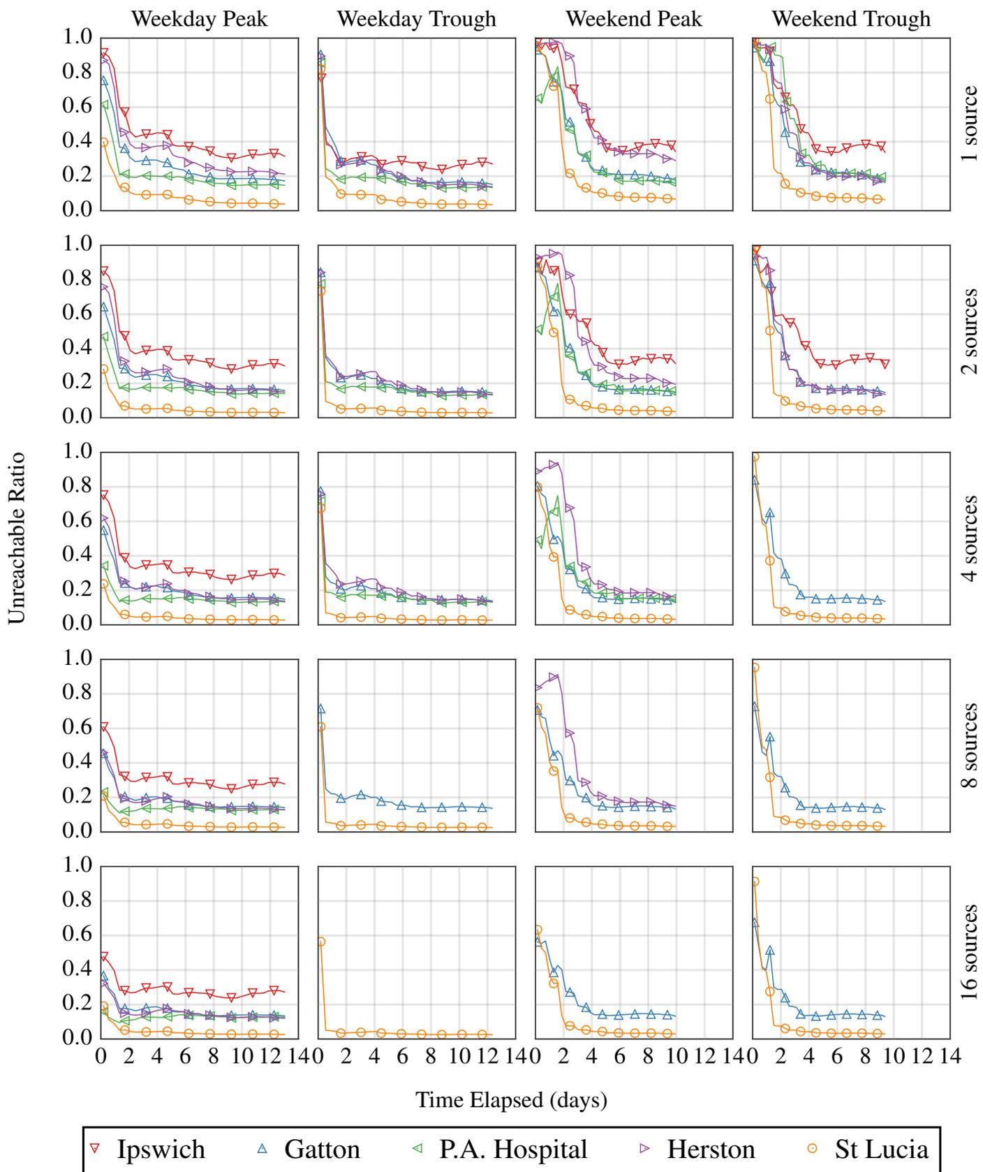
Figure 5: Unreachable ratio based on number of source devices and diffusion start time (optimistic).
