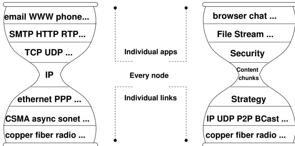
Figure 3.1: CCN replaces host-addressed IP packets, the current universal component of the network stack, with chunks of named content [1].
