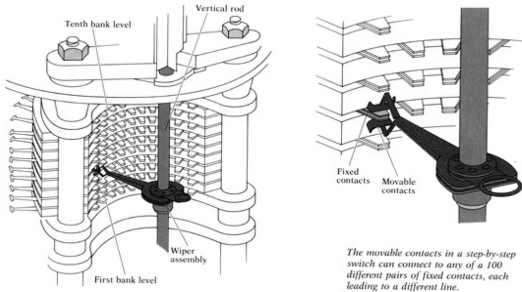
Figure 2.4: The Strowger Switch [18]—an electromechanical switching device.
