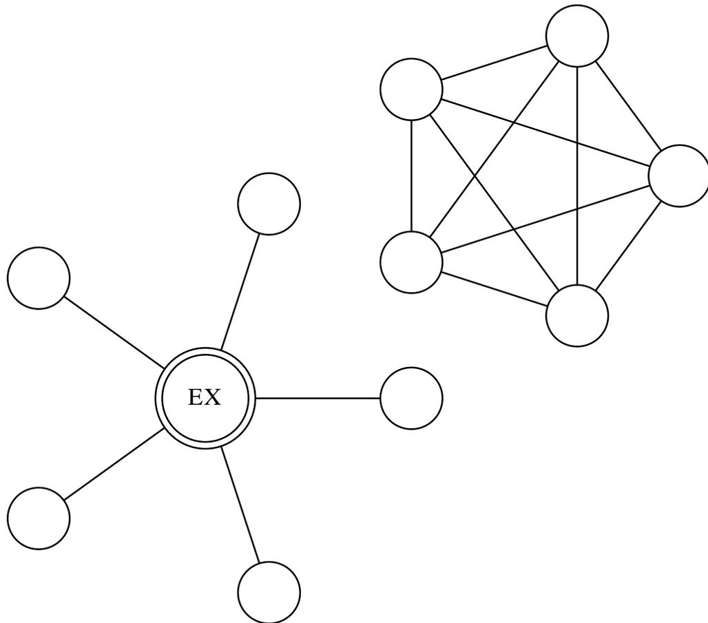
Figure 2.2: Clique (top right) and star (bottom left) network topologies. “EX” marks the telephone exchange in the star topology.
