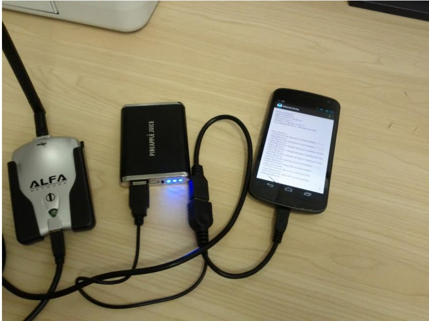
Figure B.4: A screenshot of an Android handset running *liber80211* interfacing with an external USB Wi-Fi adapter and powered via an external USB battery pack.
