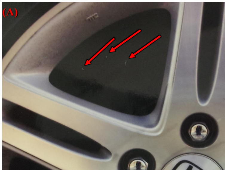
Figure 5.15: Car wheel image sample exhibiting (1) 'fingerprints visible on surface' artefact. [Not to scale].
