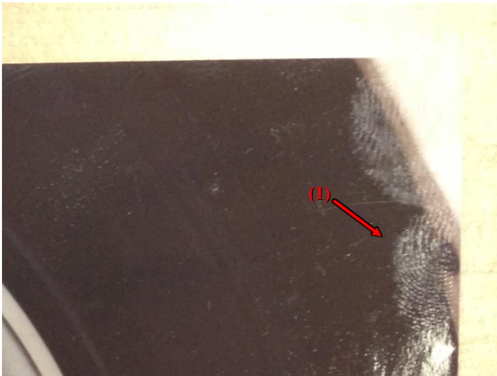
Figure 5.15: Car wheel image sample exhibiting (1) 'fingerprints visible on surface' artefact. [Not to scale].
