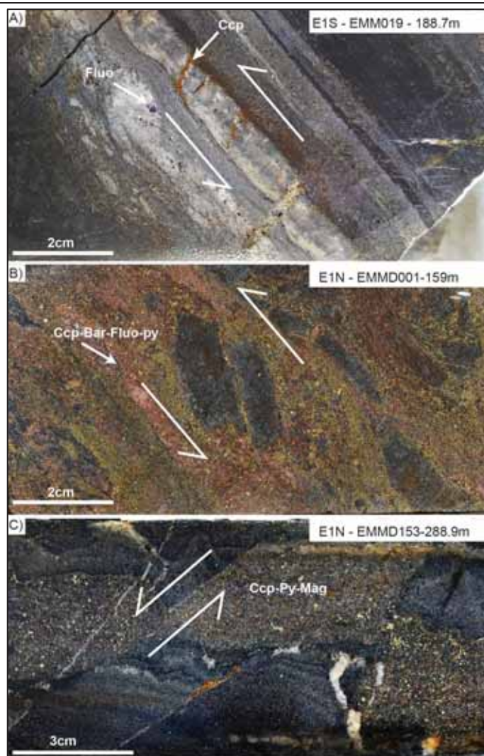
Figure 3.15: Small-scale structures. A) Boudinage of silica-rich layers in siliceous marble. Note carbonate-fluorite-pyrite-chalcopyrite veins forming boudin necks. B) Sheared metavolcanic breccia? or siliceous metasedimentary rock. Groundmass is entirely pyrite-magnetite-chalcopyrite-barite-albite-fluorite-altered. C) Dilation in magnetite-altered marble with magnetite-pyrite-chalcopyrite infill, associated with faulting and shearing? Ccp, chalcopyrite; Mag, magnetite; Bar, barite; Fluo, fluorite; Py, pyrite. The kinematic indicators are sinistral but the lack of oriented core inhibits determination of their true sense.
