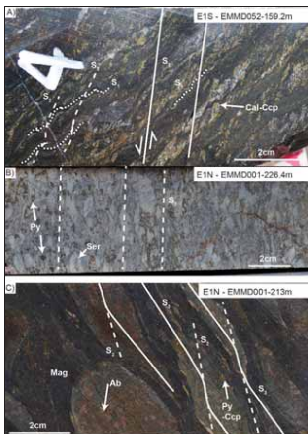
Figure 3.17: Representative deformation fabrics. A) S_1 compositional layering, or possibly S_0 / S_1 composite layering, in graphitic chlorite metasiltstone, crenulated by S_2 and S_3 . B) S_2 flattening of metavolcanic breccia clasts. Note the white haloes in clasts caused by magnetite destruction. C) S_3 shearing of S_2 -foliated metavolcanic rocks. Groundmass is mostly magnetite with blebby sulfides. Note phenocrysts in “clasts”. The magnetite may replace a S_3 shear fabric resulting in pseudobreccia in porphyritic metavolcanic rocks, or may replace a primary breccia matrix. Continued on the next page.
