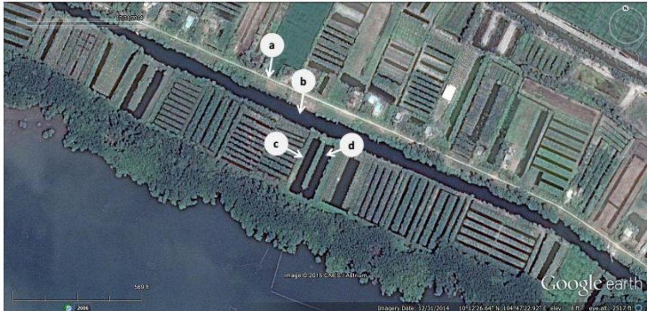
Figure 4: Typical agriculture production on private lands in Hon Dat district, a) the earth sea dyke, b) the deep channel on the sea ward side, c) crops planted on high elevation areas within ponds, and d) deep channels within ponds to store fresh water for irrigation. 10°12'26.64" N and 104°47'22.92" E. Google Earth . 31 December 2014. [viewed 3 April 2012].
