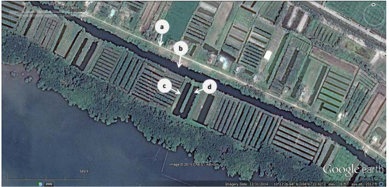
Fig 10: Typical agriculture production on private lands in Hon Dat district, a) the earth sea dyke, b) the deep channel on the sea ward side, c) crops planted on high elevation areas within ponds, and d) deep channels within ponds to store fresh water for irrigation. Source: “Hon Dat coast.” 10°12’26.64” N and 104°47’22.92” E. Google Earth. 31 December 2014. [Accessed 25 December 2015].
