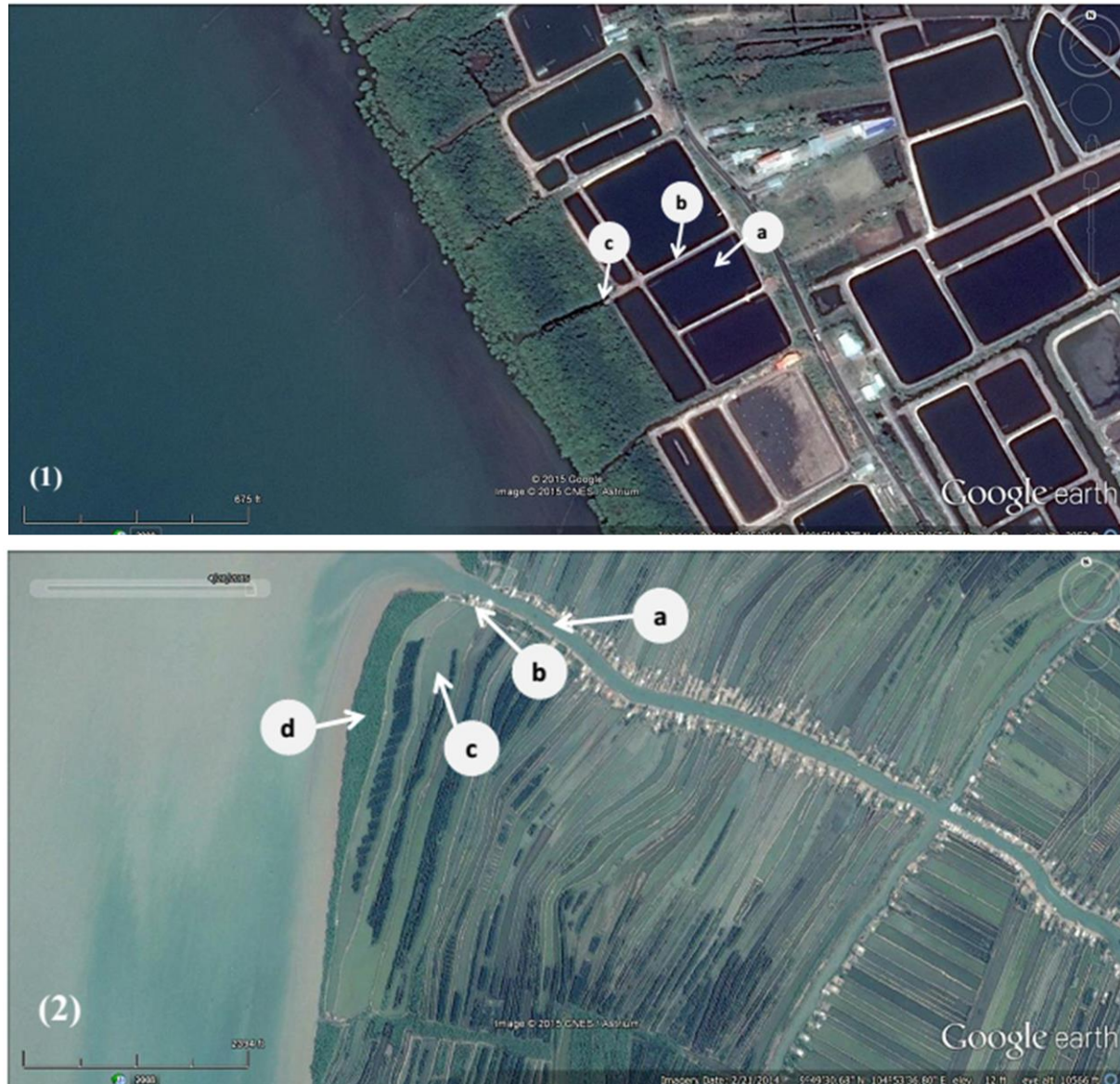
Figure 3: Two pond construction techniques have been repeatedly used over time in Kien Giang province, (1) pond construction and operation in Kien Luong district, a) pond area, b) pond dyke, and c) a pond gate was opened across the mangrove edges towards the sea to allow saline water into ponds during high tides, and were closed during low tides. 10°15'48.27" N and 104°34'37.06" E. Google Earth . 25 December 2014. [viewed 3 April 2014]. (2) pond construction and operation in An Bien district, a) natural river, b) a gate was constructed adjacent to the river to supply water to ponds, c) coastal mangrove areas cleared to construct ponds for aquaculture and d) mangrove edges. 9°49'30.68" N and 104°53'36.80" E. Google Earth . 21 February 2014. [viewed 3 April 2014].
