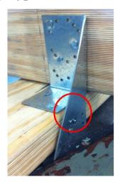
**Figure 4.5.** Defective gun nailed triple grip connection specimens: a) Type E-1, b) Type E-2, and c) Type E-3
