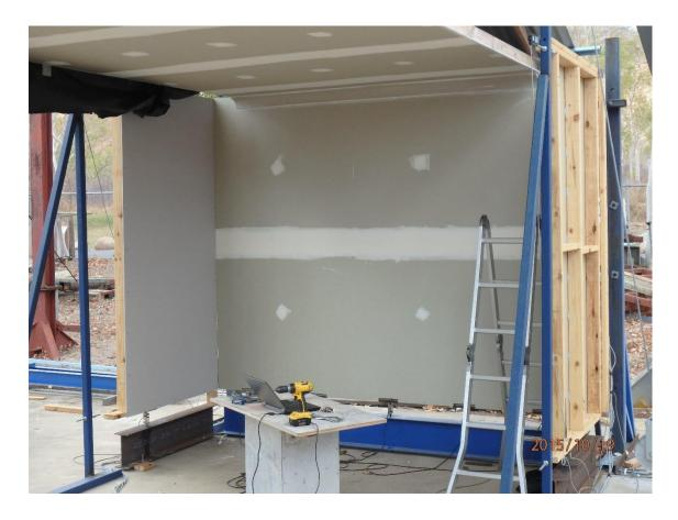
Figure B.21. Full-scale test structure with shear walls at Stage S8
