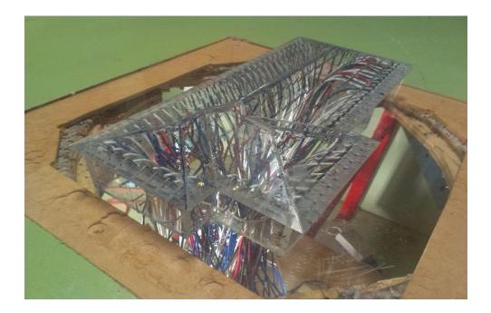
Figure 7.1. 1/50 scale wind tunnel model of representative contemporary house
