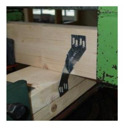
Figure 4.14. Truss grip connection test specimen
