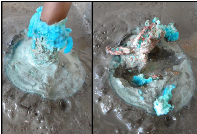
Figure 6.1 The copper anode corroded such that it consumed and disintegrated completely
