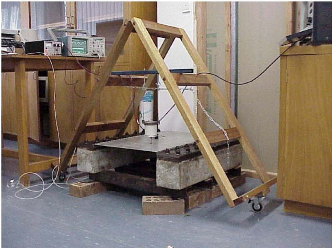
Figure 5.11 – Apparatus used to Calibrate Accelerometers
