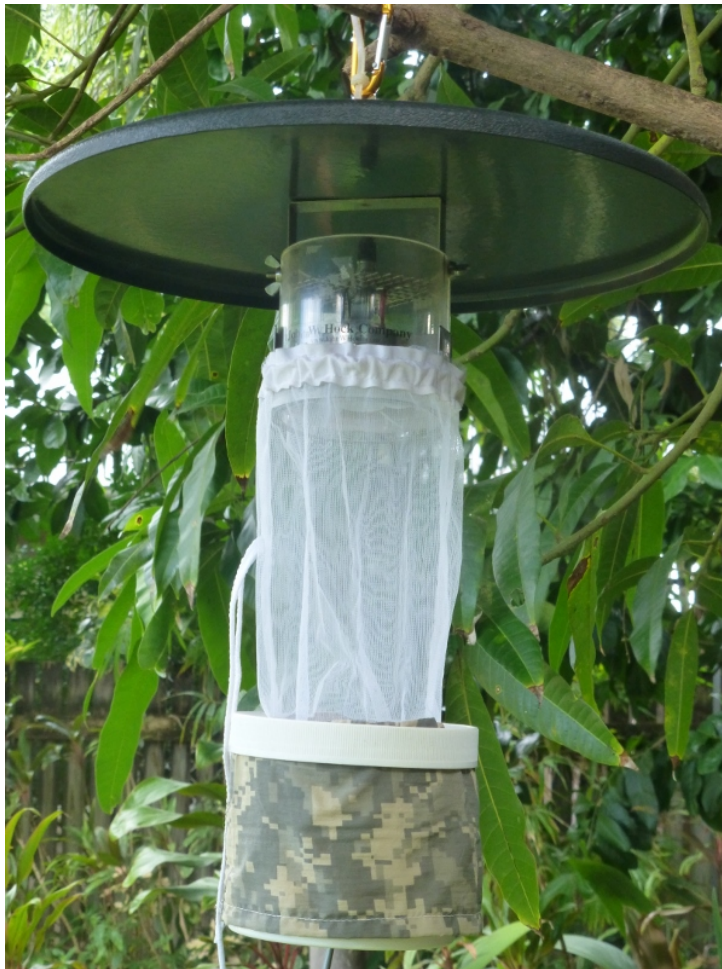
Figure 1: CDC (Center for Disease Control and Prevention) Miniature Trap Model 512 (John W. Hock Company, Gainesville, U.S.A.) used in Chapter 2 and 4.
