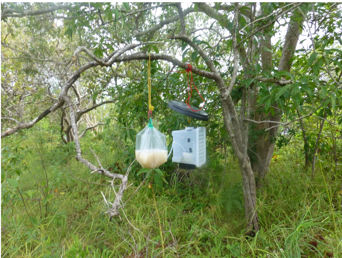
Figure 4: Non-powered passive box trap in combination with CO 2 produced by yeast and sugar fermentation used in Chapter 5 on the islands of Saibai, Boigu, Badu and Moa.
