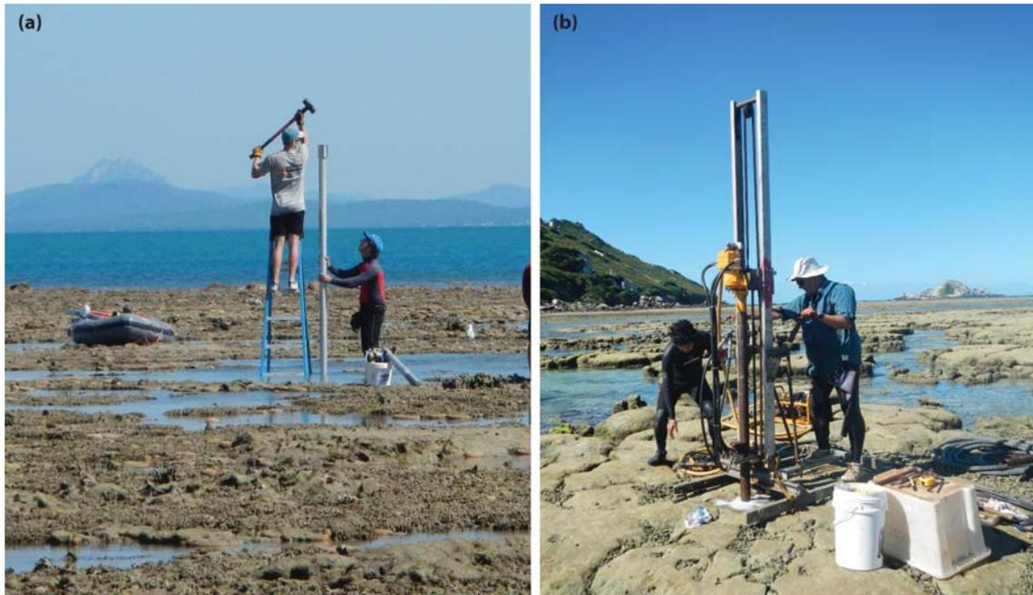
Figure 1.4 (a) Percussion coring on the reef flat at Middle Island; (b) rotary drill rig set up on a fossil microatoll at Holbourne Island flat.
