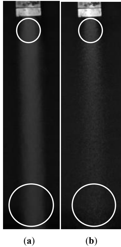
Figure 5.13: Visible images of the particle curtain showing the sparsity of particle at on the top and bottom of the curtain (a) d_s=290\mu\text{m} , m^o=0.14\text{kg/s} and slot width=20mm (b) d_s=610\mu\text{m} , m^o=0.088\text{kg/s} and slot width=20mm
