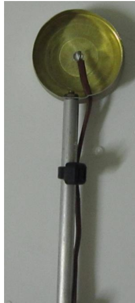
Figure 4.13: The sampling cup fitted with a T type bead thermocouple
