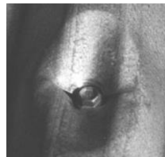
Figure 1.2: Static pull-through failure (credited to: Mahaarachchi, 2003)
