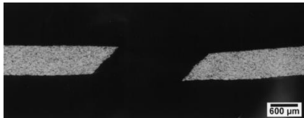
Figure 2.33: Fracture plane through the thickness of sheet metal subject to out-of-plane biaxial stretching (credited to: Jain et al, 1999)
