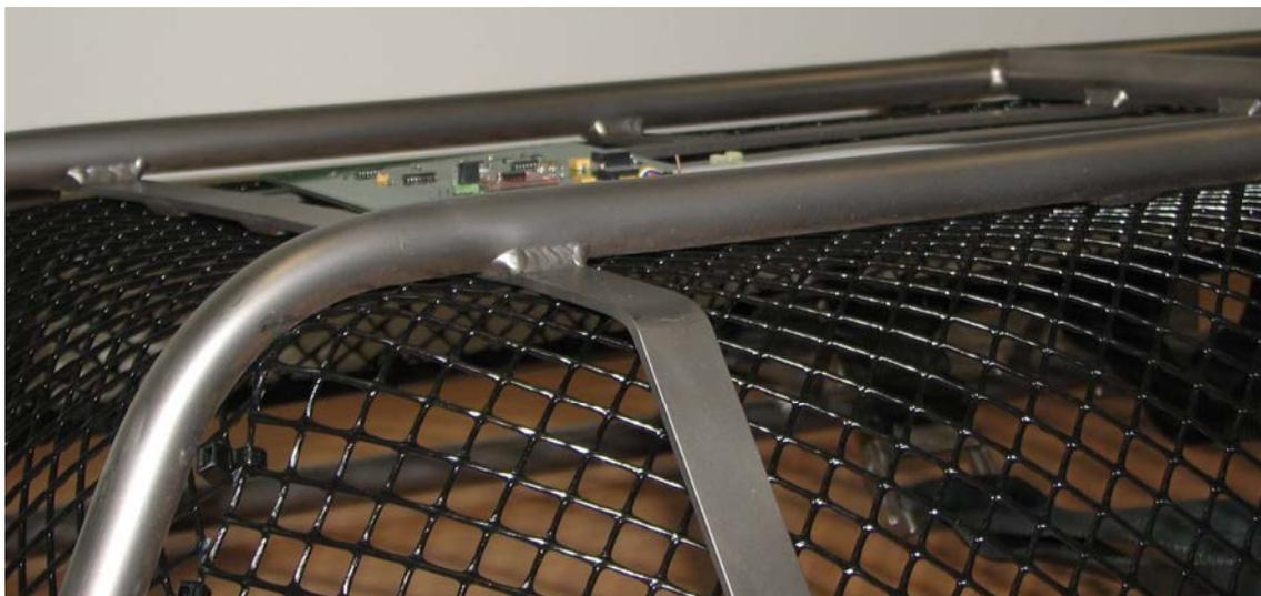
**Figure 3.2:** Shows the cavity beneath the litter created by the 19mm tubular frame. Note that in this image the litter is inverted. Due to its lightweight construction the litter frame suffers considerable flexing during handling particularly when held from the ends as it is when the litter is being manoeuvred into the helicopter.
