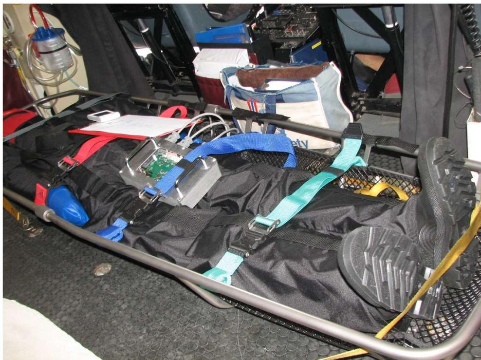
**Figure 4.7:** Showing the rescue litter and mannequin positioned in the helicopter. The litter is placed across the floor directly behind the pilots seats which are at the top of the picture. The mannequin is restrained in the litter with the red, blue and green belts and the litter is restrained in the helicopter by the yellow belts at each end.
