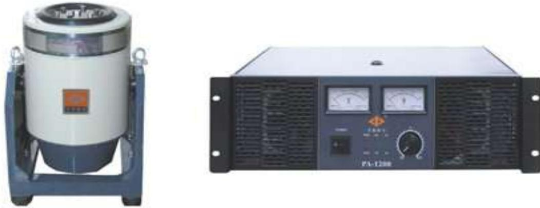
**Figure 5.1:** Dongling ESS-050 500 Nt shaker (left) and PA1200 amplifier (right). The moving shaker core is the disk with five attachment bolts inside the rubber seal on top of the shaker.
