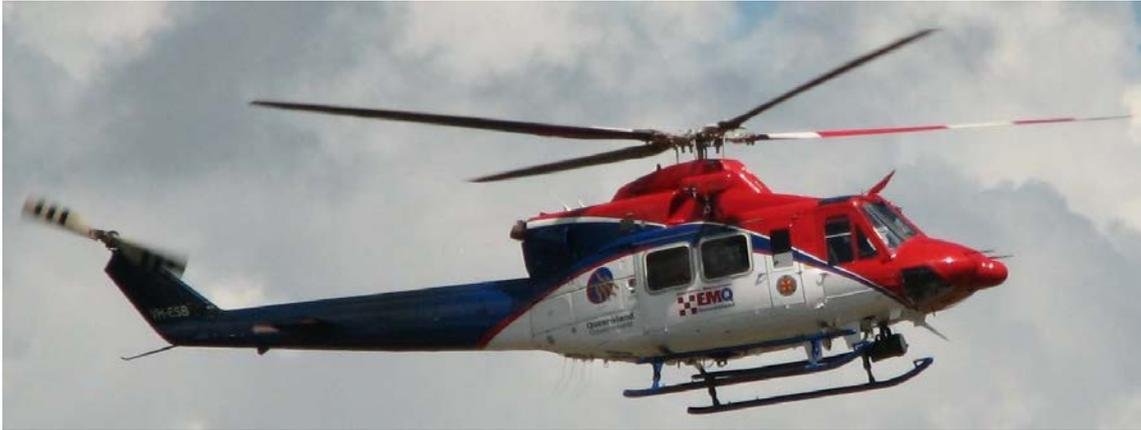
**Figure 2.0:** Emergency Management Queensland (EMQ) Bell 412 is typical of the rescue helicopters used for retrieving DCI patients from the Great Barrier Reef to The Townsville Hospital. Note the winch above the sliding door in line with the main rotor vertical shaft. The sliding door can be identified by the double large square windows.
