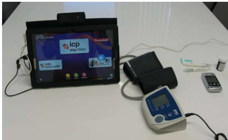
Figure 4-1. The in-home monitoring device of the clinical trial- a tablet pc, sphygmomanometer and a glucometer.
