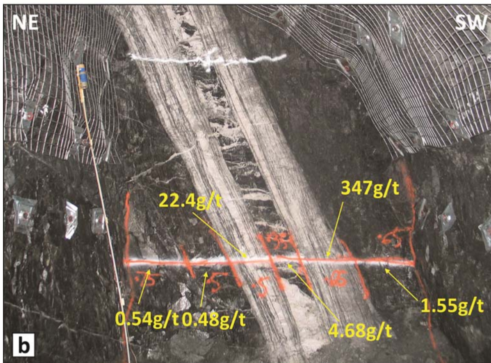
Figure 7.7 – Underground face photographs of the Raleigh vein with face sample intervals for scale (red numbers in metres) and assayed gold grades (yellow: grams per tonne, or ppm Au); a) the ore is contained in a 1-2 m thick laminated quartz-carbonate vein emplaced within a thin metasedimentary unit at a contact between andesite and gabbro; b) bonanza grade, strongly laminated quartz carbonate vein with a large inclusion of rock and extensional veins that may be a preserved remnant of the original extensional shear vein array, progressively sheared to form the finely banded quartz/wallrock ribbon vein. Photos from Placer Dome underground mine face documents (R. Hutchison written communication 2006).
