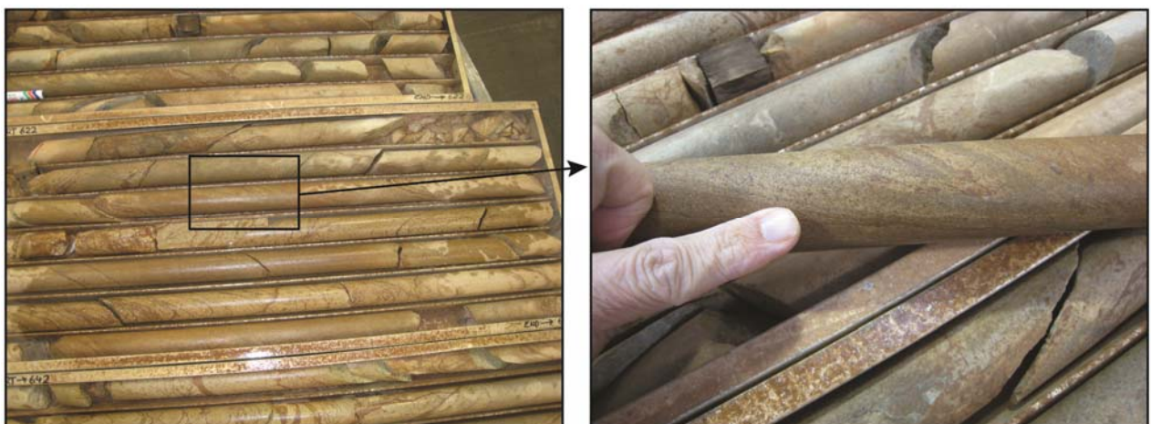
Figure 4.6 – Flow-banded dacite sample SG16482 from 186.6 m-193.2 m (622 ft - 644 ft) in Western Mining Corporation drill hole SE3.
