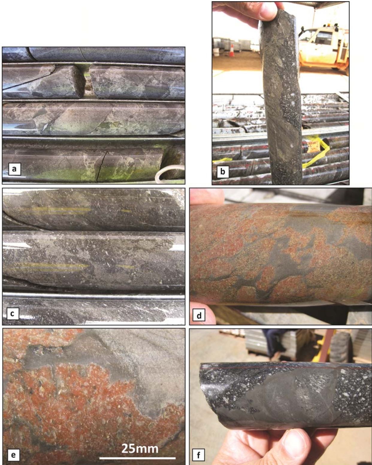
Figure 3.18 - Typical examples of lower Black Flag formation rocks correlated with the Binduli sequence in Kundana South drill core (50 mm diameter). a) Angular felsic breccia/conglomerate, with cusped volcanic clasts, GOLD07-921 160 m - GDA: 334348E; 6597467N; b) Sharp intrusive contact of porphyry with bedded sandstone, GOLD07-993 222.2 m - GDA: 335122E; 6596670N; c) Amygdaloidal crystal-rich volcanic hyaloclastite, GOLD07-993 446 m, d) Peperitic margins of feldspathic volcanic rock, GOLD07-907 220 m - GDA: 334416E; 6598105N, identical to rocks recorded at Binduli by Doyle (1999); e) Peperitic margins of feldspathic volcanic rock, GOLD07-907 220 m, f) Fractured feldspar porphyry with infilling by siltstone GOLD07-903 - GDA: 334912E; 6597974N. Drill cores have 50 m diameter.
