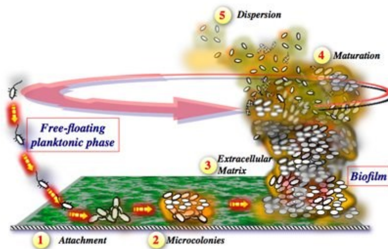
Figure 1.11 : Diagrammatic representation of biofilm formation. 1 - Attachment, 2 –Micro colonisation. 3 – The development of an extracellular matrix. 4, 5 – Maturation and dispersion of the biofilm.
