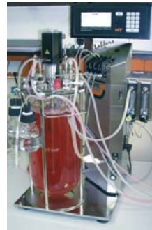
Fig 2. Cultivation of R. glutinis in fermenter batch-mode, incubated with 5% CH 4 in air.
