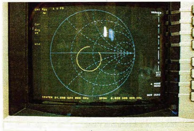
Figure 4.9 The transmission  $S_{21}$  Q-circle is much less effected by the frequency dependence of delay in transmission lines than for reflection ( $S_{11}$  or  $S_{22}$ ) circles.
