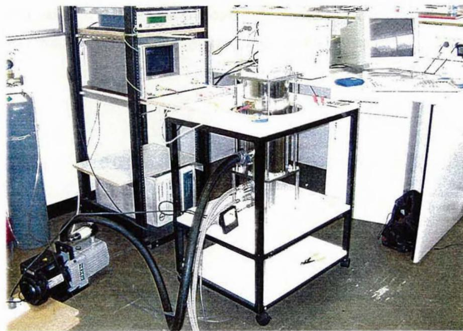
Figure 6.6 Photo of the main measurement system used in this thesis, showing the HP8722C network analyser, temperature controller, vacuum dewar with the cold head, IBM-PC computer, and rotary vacuum pump. The compressor of the cryocooler system is not visible in the photo.
