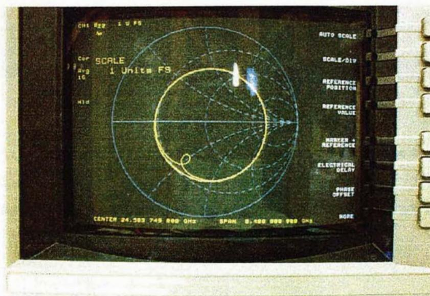
Figure 4.10 Mismatch effect observed in the off-resonance part of the reflection  $S_{22}$  trace. The  $S_{22}$  Q-circle (which is evidently distorted due to transmission line phase effects) is attached to the relatively larger off-resonance circle. The centre of the off-resonance circle clearly does not coincide with the centre of the Smith Circle, indicating the presence of impedance mismatch.
