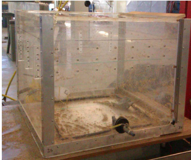
Figure 4. 3 : The Perspex tank used in the settlement tank test
