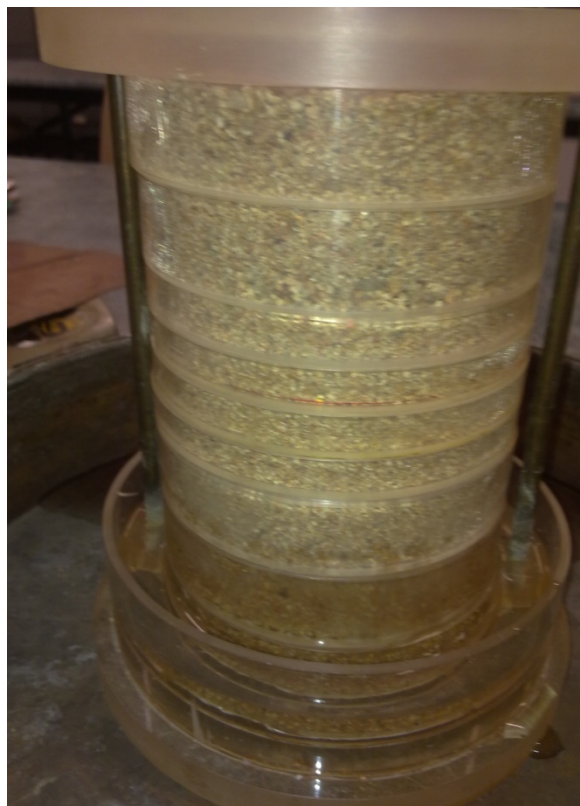
Figure 4. 11 : Capillary test of sieved soil using Perspex tubes protruding from water
