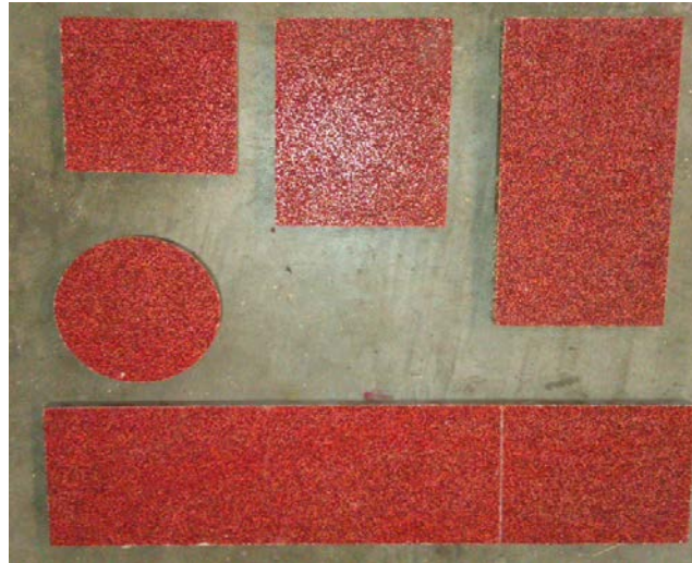
Figure 4. 4 : Model footings used in the settlement tank test
