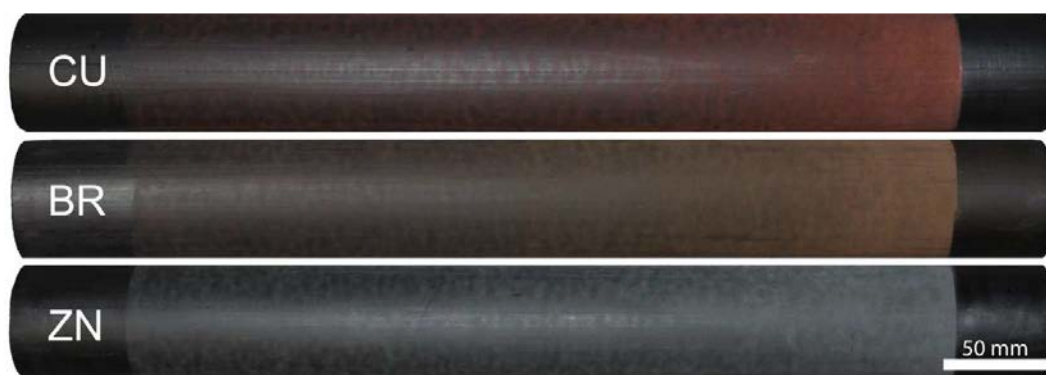
Figure 6.1. Black HDPE tubes embedded with copper (CU), bronze (BR) and zinc (ZN) metal particles (< 50 \mu\text{m} diameter) using cold spray technology. Particles vary in loading density from low (left) to high (right) along their lengths and only the middle 400 mm of the 500 mm tube was sprayed.
