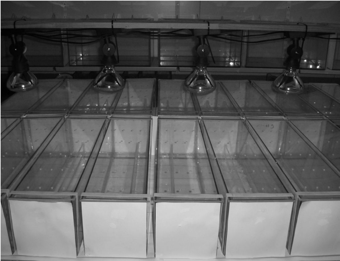
Figure 7.1. The thermal gradients used during this experiment. Each thermal gradient consisted of a glass aquarium (60 × 15 × 15 cm) with a heat lamp positioned above one corner, and allowed each frog to select body temperatures ranging from 20°C at the cool end to 30-50°C at the warm end, depending on the frog's rate of evaporative water loss.
