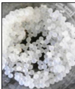
Fig.7.5 Immobilized TiO 2 -gel beads
