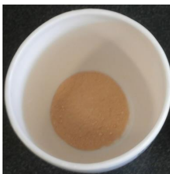
Fig.7.3 Synthesized TiO 2 /zeolite from acid-alkali activated zeolites after oven drying (before homogenisation)
