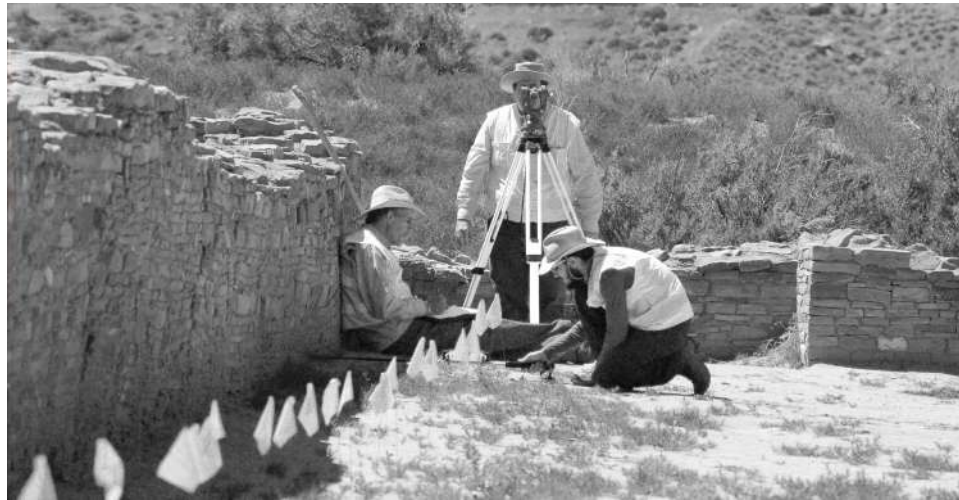
Figure 48. Survey of Pueblo Bonito's NS bisecting wall
