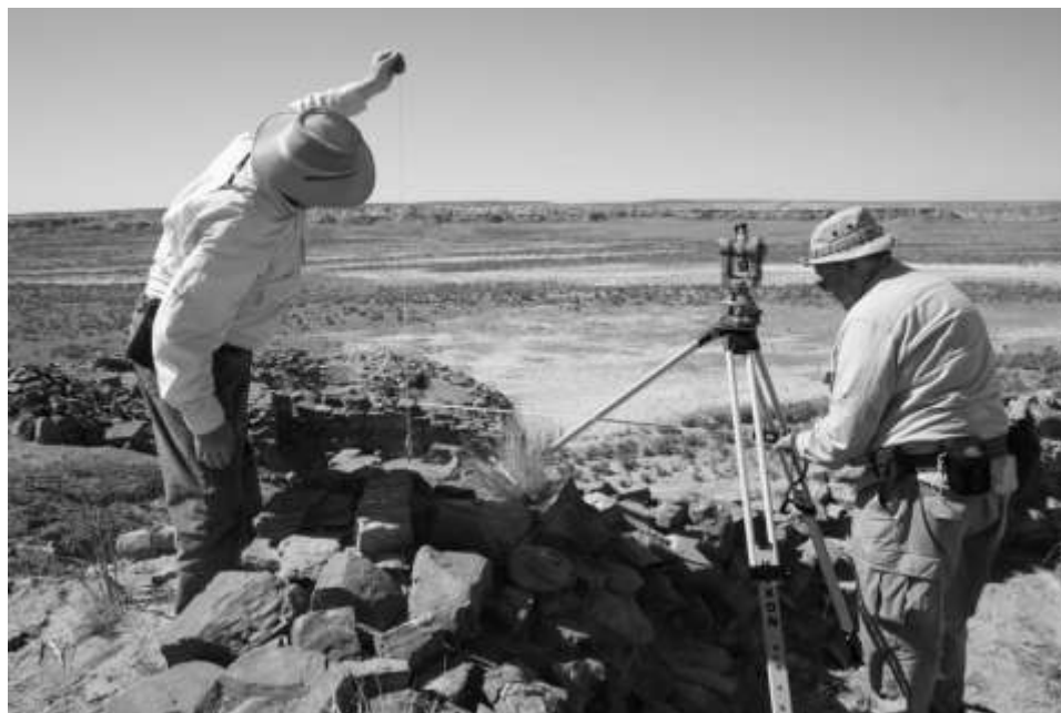
Figure 93. Theodolite setup at Bis sa'ani east room block
