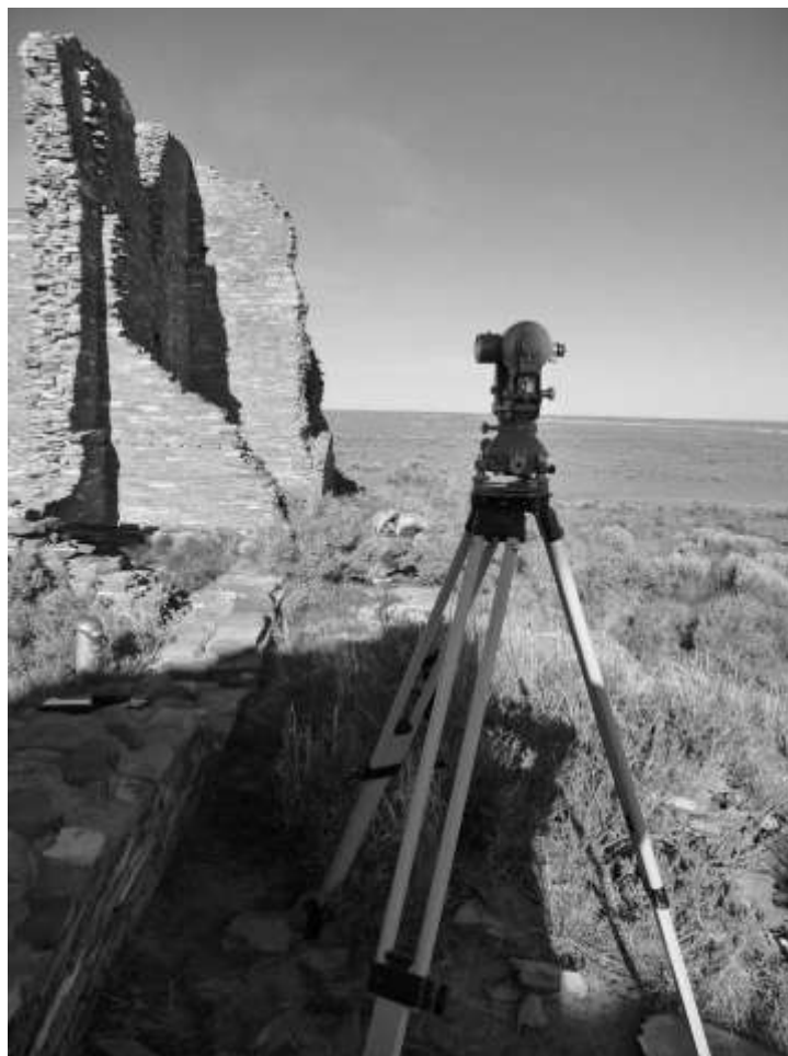
Figure 102. Theodolite survey of Pueblo Pintado's west wall
