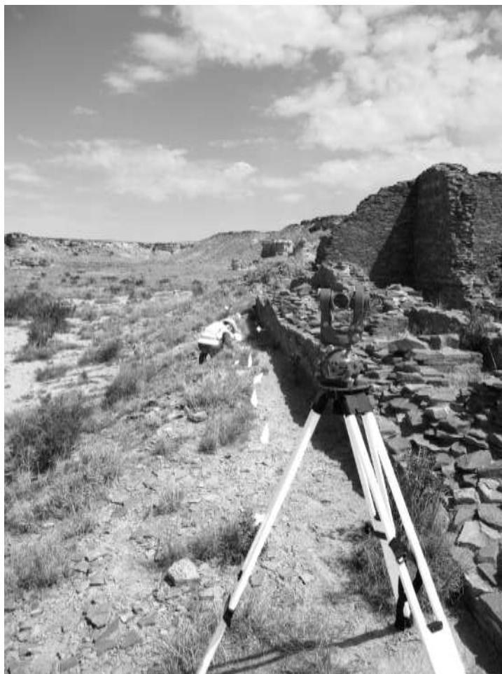
Figure 100. Theodolite survey of Kin Bineola's west wall
