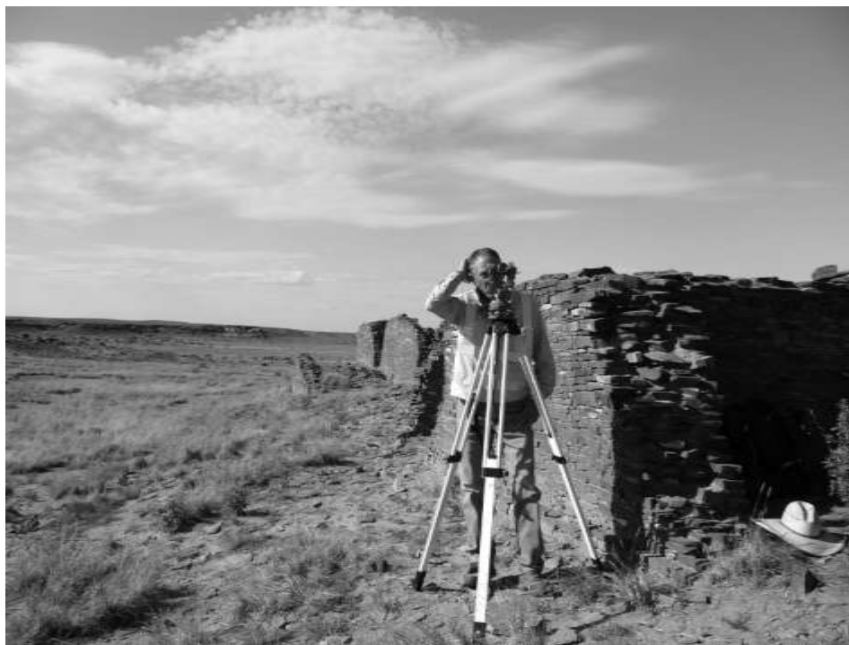
Figure 99. Theodolite survey of Kin Bineola's east wall
