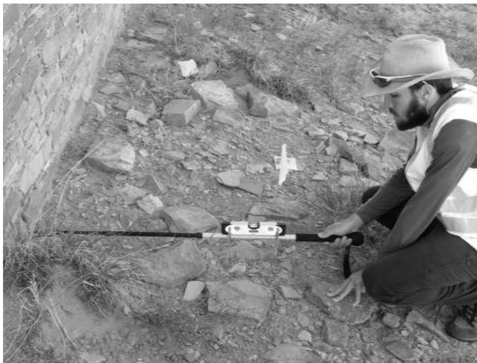
Figure 25. Improved angle measurement technique for walls
