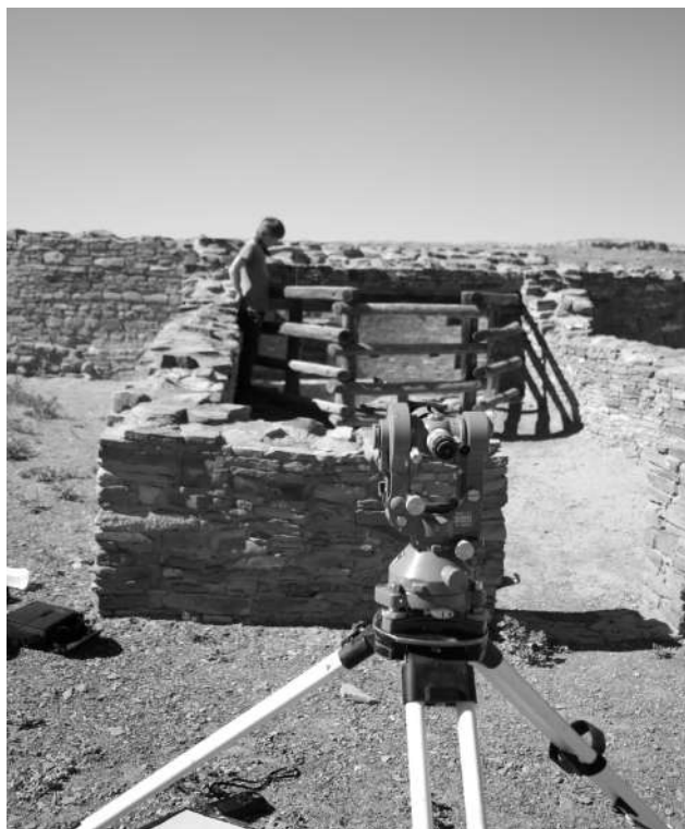
Figure 58. Theodolite survey at Casa Rinconada
