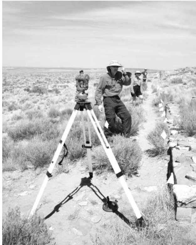
Figure 62. Theodolite survey of Pueblo Alto's north wall, west section
