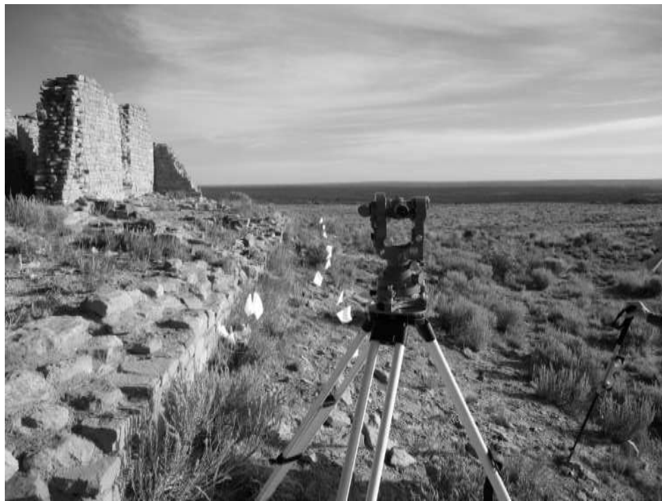
Figure 59. Theodolite survey of New Alto's east wall
