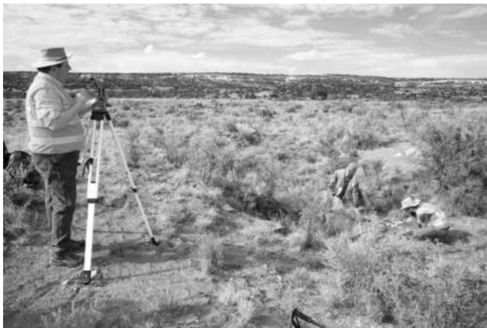
Figure 79. Theodolite survey of Shabik' eshchee's pithouse B deflector Among the surrounding pithouses, only this site had adequate above ground exposure to enable survey.
