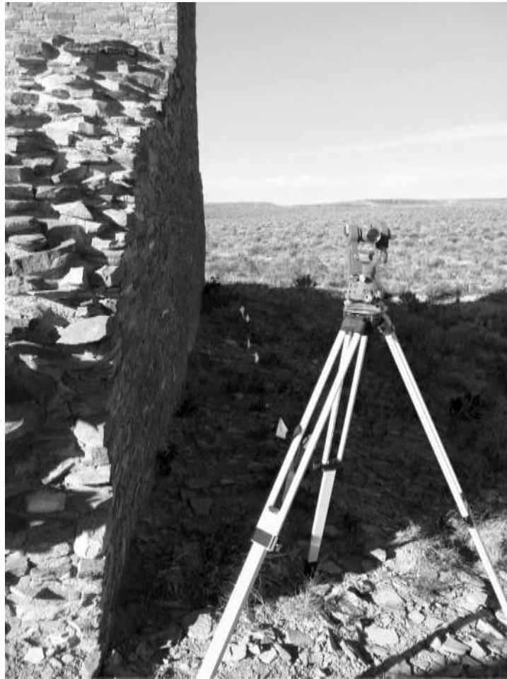
Figure 97. Theodolite Survey of Kin Klizhin's back wall
