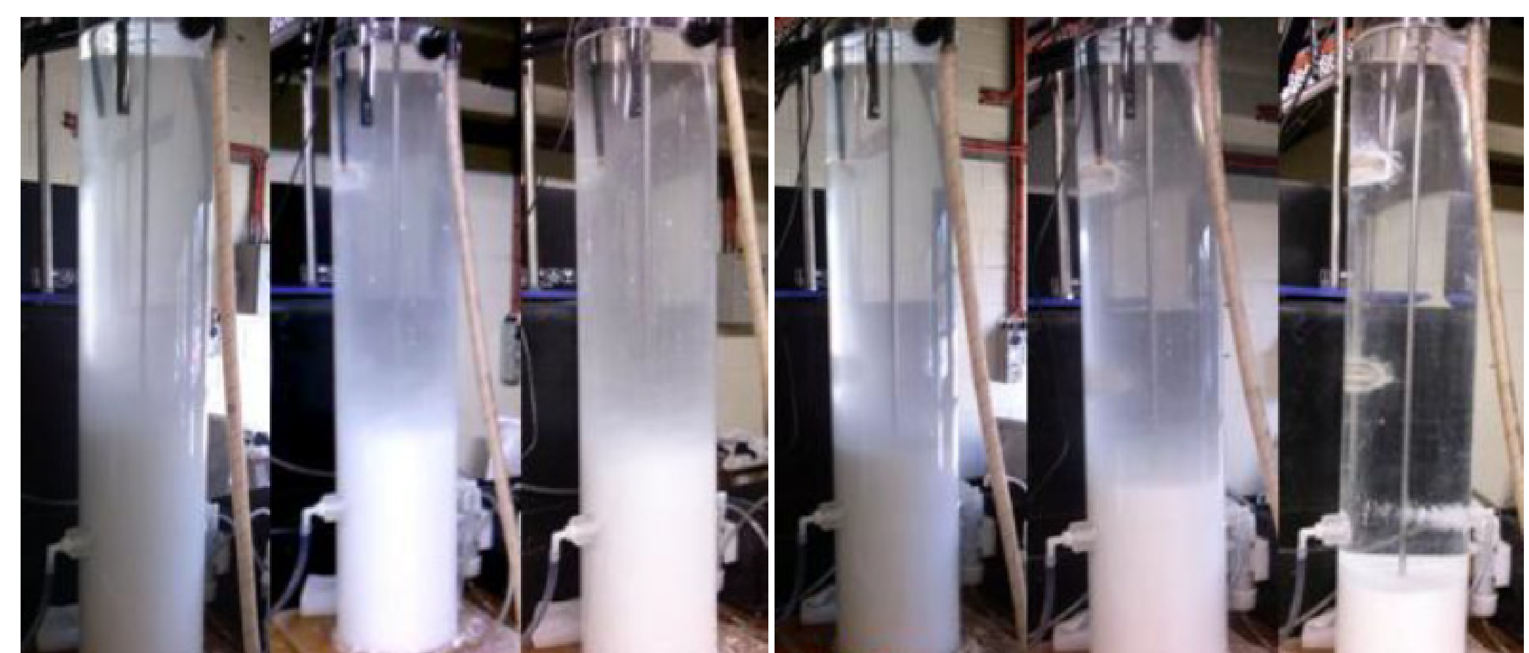
Figure 2: Operating nutrient recovery reactor showing bed height reduction throughout the recovery campaign
