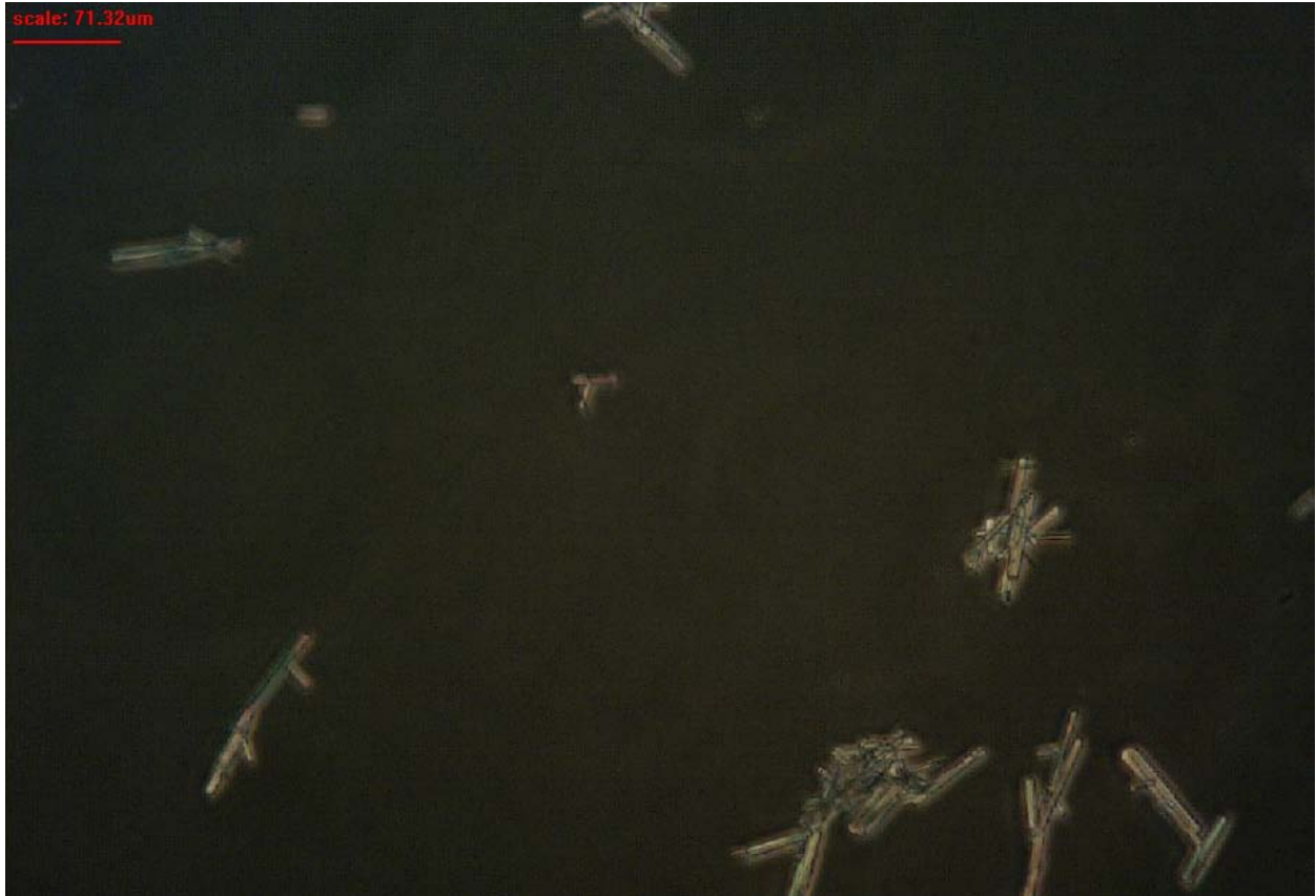
Figure 6.5: Struvite crystals produced using the experimental procedure developed for this work.
