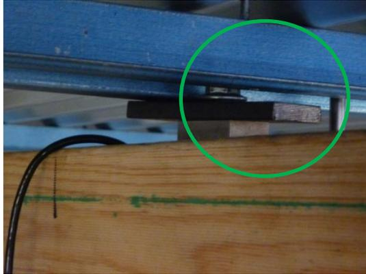
Figure 5.28: Batten-to-Truss connection with one screw connection removed
