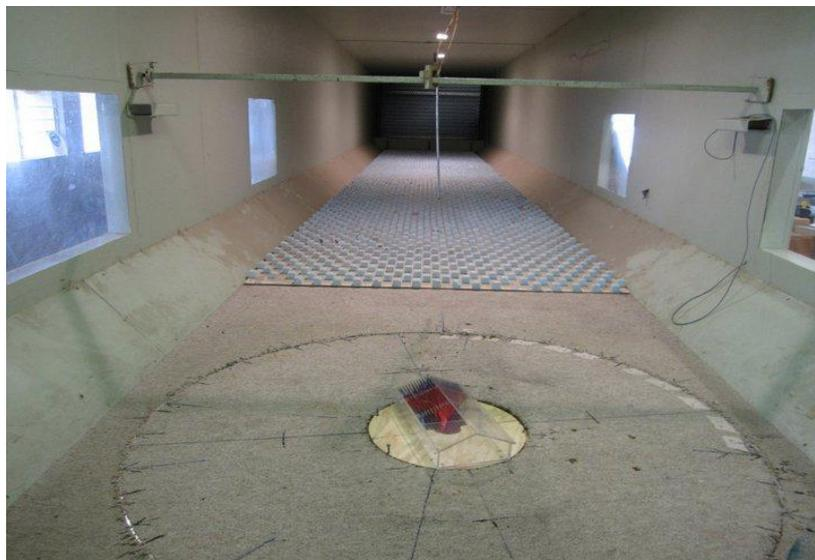
Figure 4.5: 1/50 scale model of the 10m x 19.8m x 2.7m house in the wind tunnel
