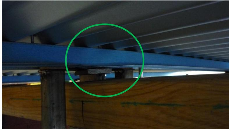
Figure 5.35: Plastic deformation of a batten-to-truss connection
