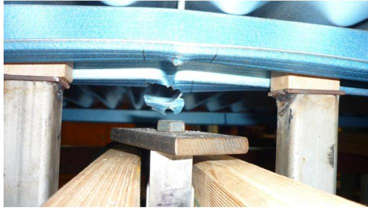
Figure 5.37: Failure of the connection (b2, R2)
