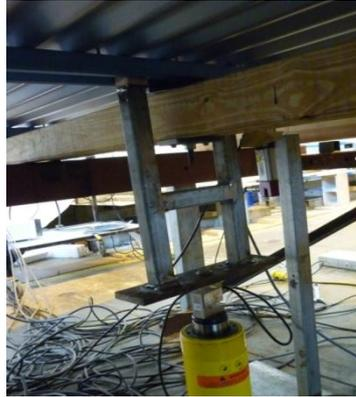
Figure 5.31: Applied load on batten-truss connection
