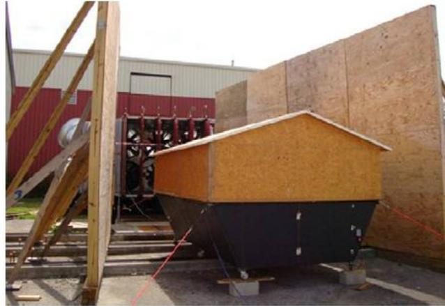
Figure 2.3: 1/3 scale model building (Mensah *et al.* (2011))
