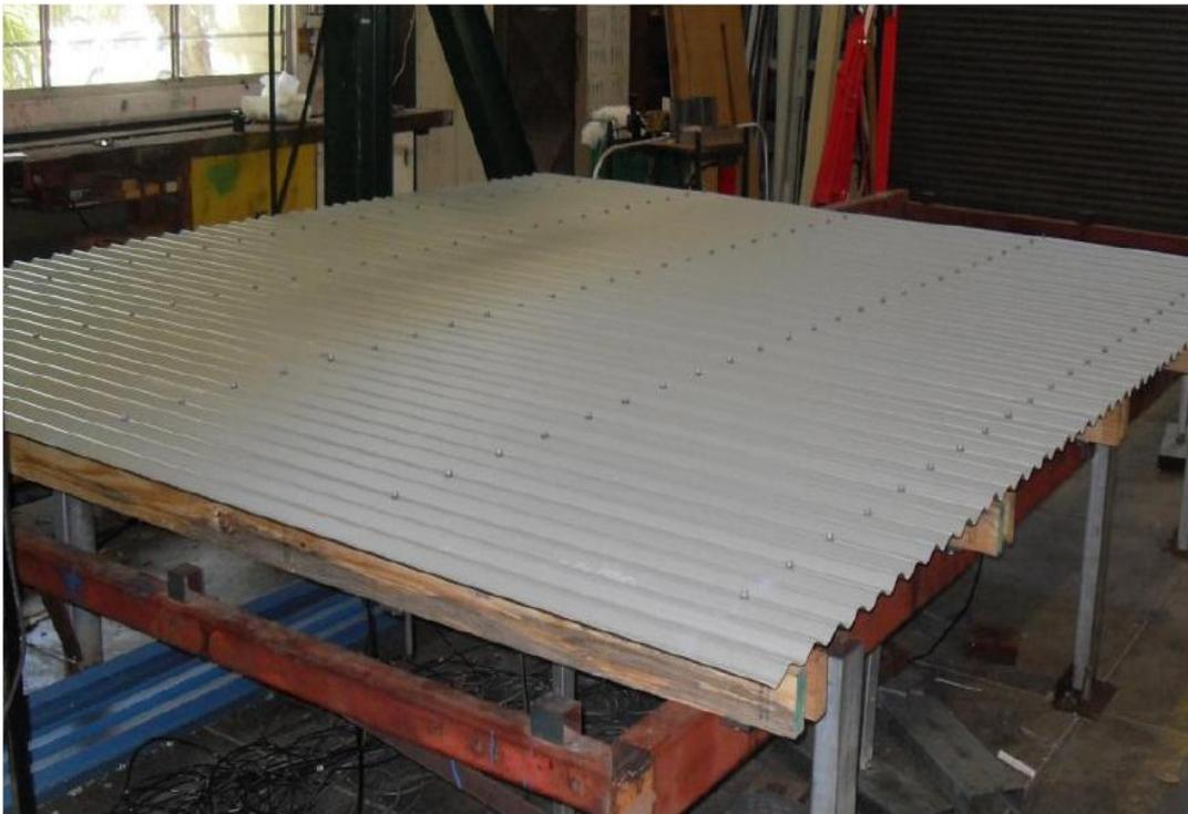
Figure 5.5: Test set up with cladding fixed
