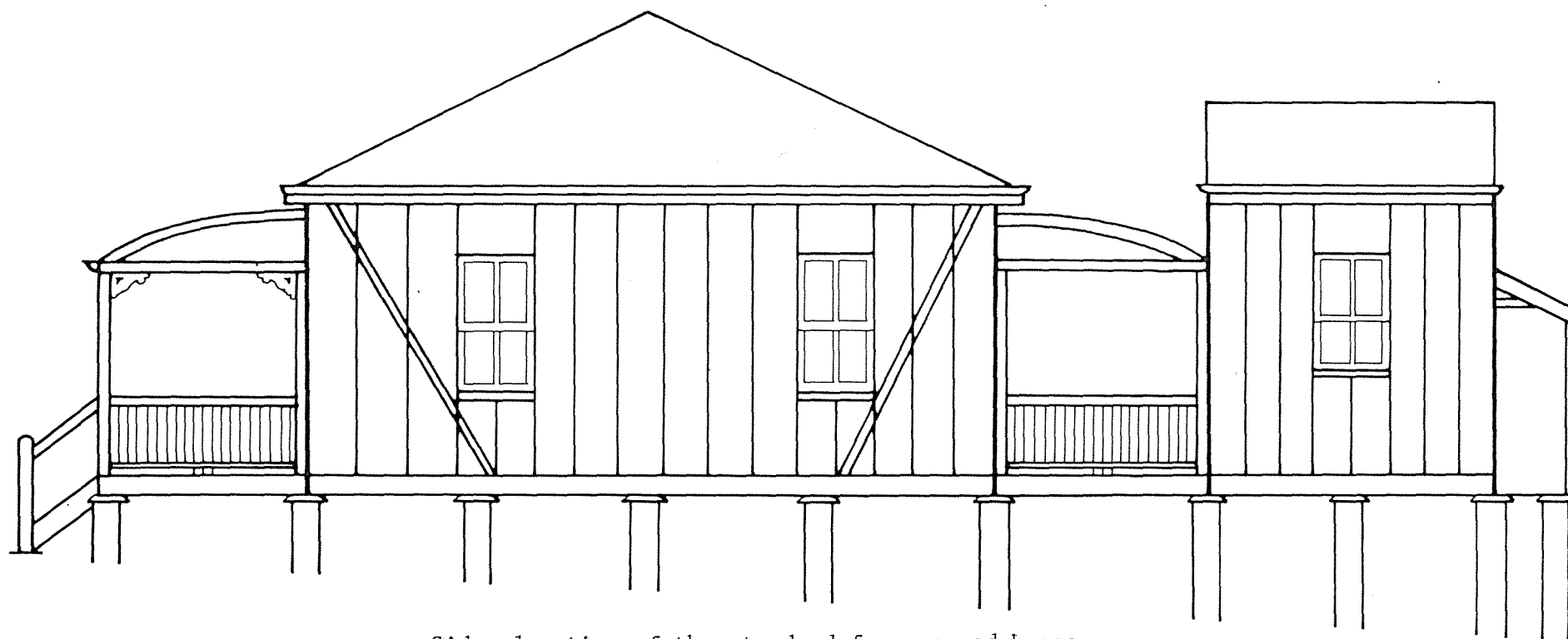
Side elevation of the standard four-roomed house
