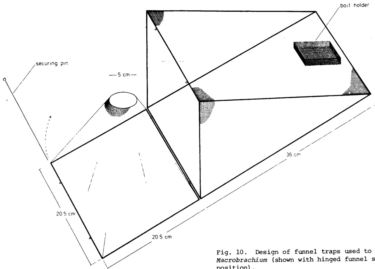
Fig. 10. Design of funnel traps used to sample adult *Macrobrachium* (shown with hinged funnel section in open position).
