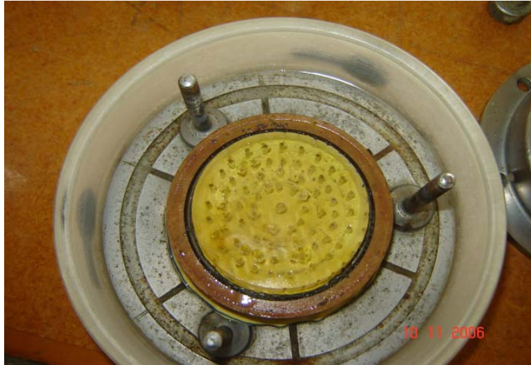
Figure 5.7 One side drainage in oedometer
