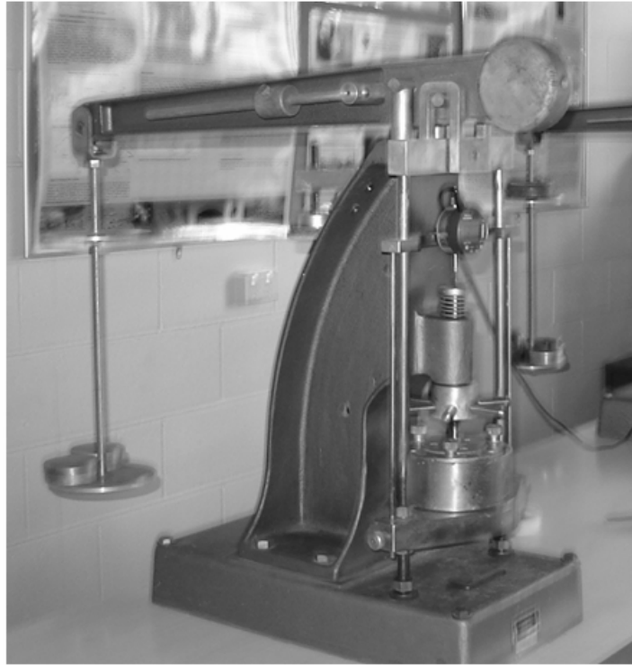
Figure 5.5 Conventional oedometer apparatus
