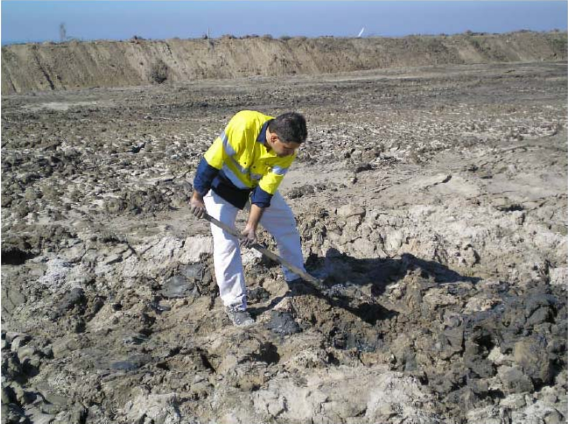
Figure 4.4 Shoveling method was conducted for sampling in the paddock of S3b
