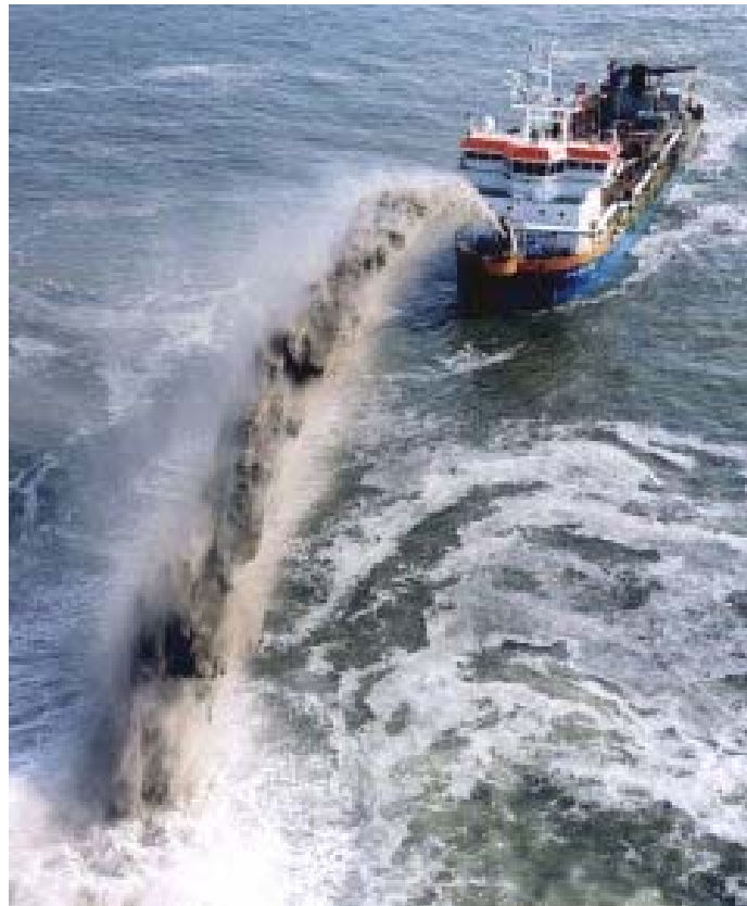
Figure 2.20 Discharging method for high moisture content slurry
