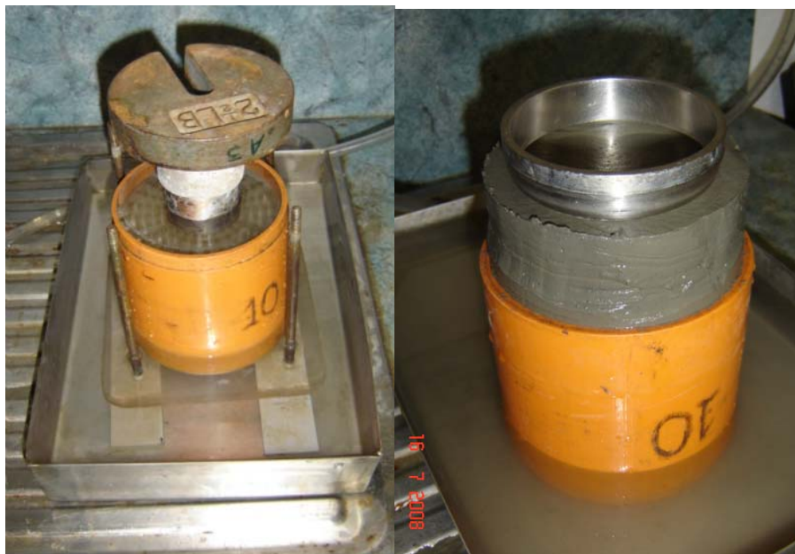
Figure 6.1 Preparation and recovering of a sample for oedometer test
