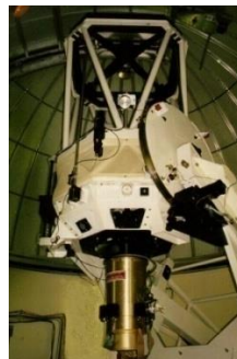
FIG. 3.3- The three-band NIR camera (gold colored cylinder) mounted on the 2MASS telescope at Mt. Hopkins. Image taken from http://pegasus.astro.umass.edu/
