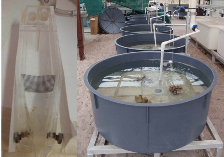
Fig 2.2 Two-channel flow chamber used for olfactory trials (left); Outdoor test aquaria for overnight habitat choice experiments each containing portions of hard coral ( Pocillopora damicornis ), soft coral ( Sarcophyton spp ), and coral rubble.
