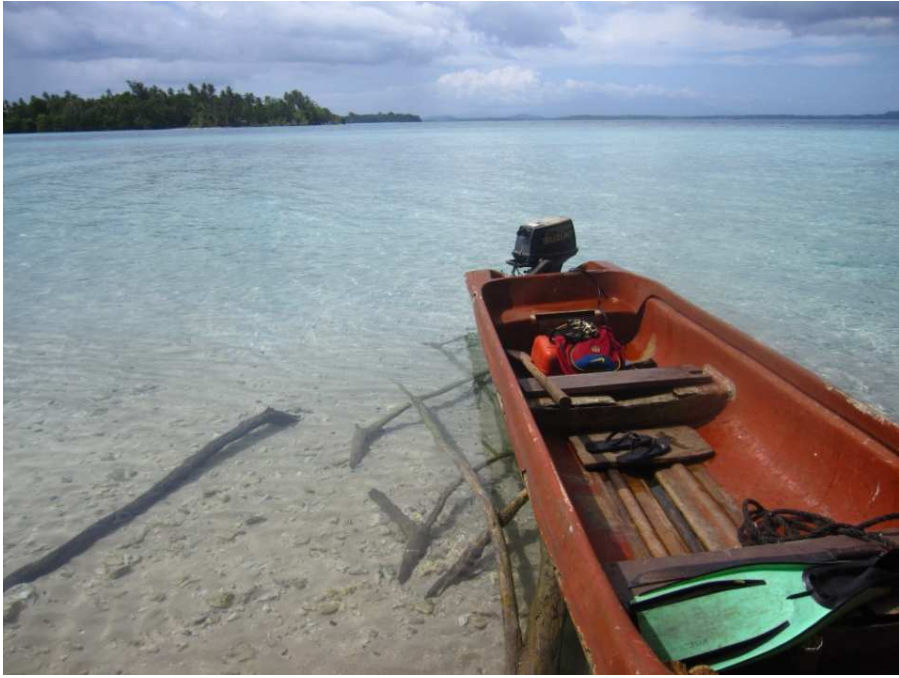
Photo 2A.2 A typical fibreglass boat used for fishing and transport throughout Solomon Islands. Most are roughly 5 -7 metres in length, equipped with a 6-15 horsepower engine. They require significant financial outlay and are costly to run due to local fuel and fibreglass costs, as well as outboard maintenance, but far more efficient and stable than dug-out canoes. This particular boat belonged to Michael Giningele, the father of Joe, who assisted with the field work for this thesis.
