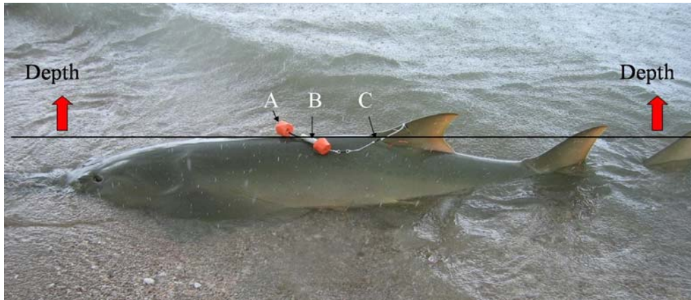
Figure 27: Position and size of acoustic tag and floats. A = LTD_10, B = acoustic tag, and C = galvanic time release. Horizontal line and arrows indicate where water depth was measured.
