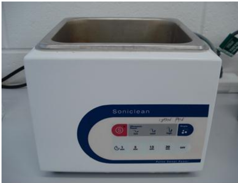
Plate 3.2: Soniclean™ 160HT ultrasonic cleaning bath used to clean deposition substrate
