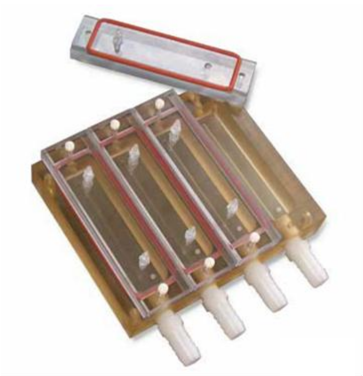
Plate 2.4: A commercially available drip flow reactor Model DFR 110 from BioSurface™ Technologies Corp. Reactors like this one provide sealed chambers with removable surfaces and use gravity to feed fluid through the chambers providing shear and drag
