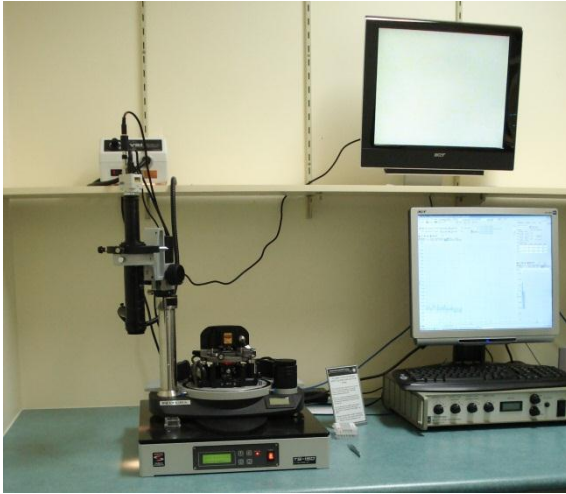
Plate 5.6: NTEGRA™ NT-MDT Prima Atomic Force Microscope at the Advanced Analytic Centre, James Cook University
