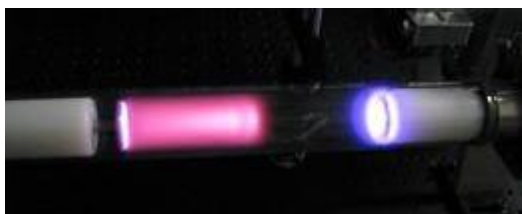
Plate 2.1: Example of visible glow produced by photons emitted from plasma generated with a glass laboratory tube reactor
