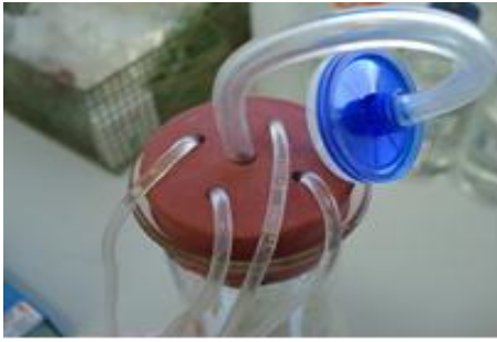
Plate 5.2: Tailored rubber flask stopper housing fluid extraction channels and a filtered air channel fitted with a syringe filter
